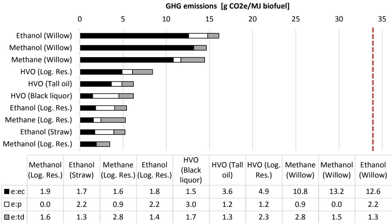
**Figure 3.** GHG emissions of extraction and cultivation efforts (e:ec), production and conversion of feedstock (e:p) and transportation and distribution (e:td) according to the EU RED methodology for the biofuels methanol, methane, ethanol and HVO with different feedstock and conversion pathways. The dashed line indicates GHG emissions of 34 g CO<sub>2</sub>e/MJ biofuel, corresponding to a 60% GHG emission saving compared to fossil fuel reference used in the EU RED.
