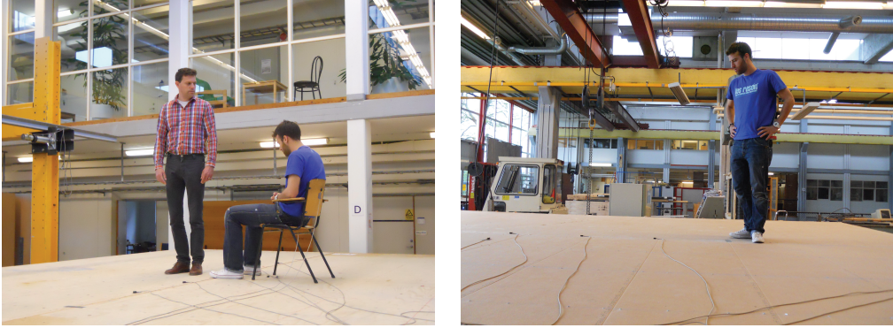
Figure 14: Measurement pictures showing the seated (left) and the walking (right) subtest.
