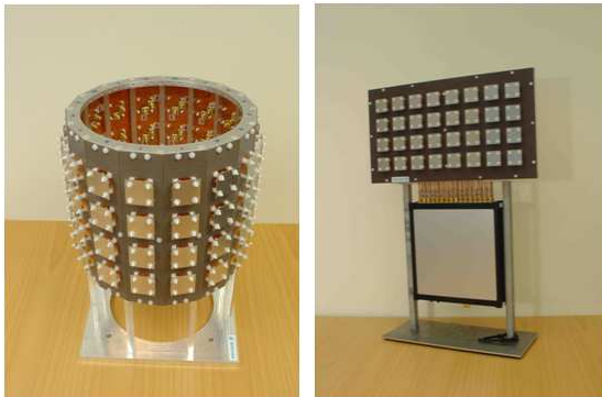
Figure 4: Receive antenna array (left) and transmit antenna array (right).
