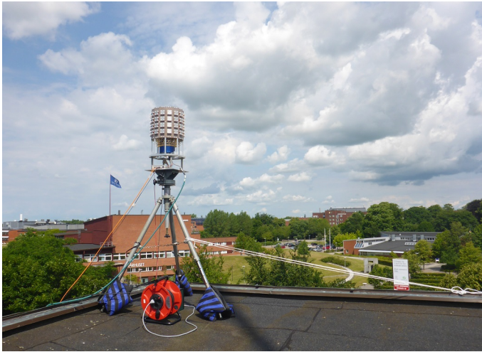
Figure 3.3: The cylindrical array on a building roof at Lund University.
