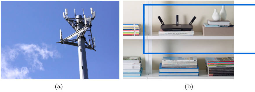
Figure 1.1: Examples of MIMO technology used in our everyday life. (a) A cellular base station tower with multiple antennas. (b) A Linksys wireless router with multiple antennas (source: www.linksys.com ).
