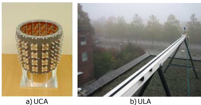
Figure 1: Two large arrays at the base station side: a) a UCA with 64 dual-polarized patch antenna elements, giving 128 ports in total, and b) a virtual ULA with 128 vertically-polarized omni-directional antennas.
