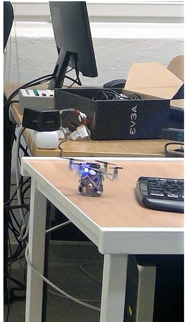
Fig. 1. The figure shows the final Crazyflie 2.0 quadcopter, outfitted with both structure that both holds the camera in place, and protects it from breaking when colliding.
