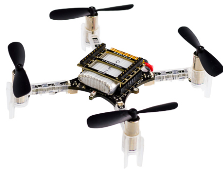
Fig. 1. The quadcopter used in this project. The Crazyflie 2.0 by Bitcraze.
