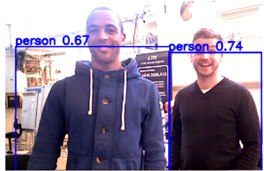
Fig. 11. The figure shows the classification done by the YOLO9000 network using an ASUS Xtion camera. The bounding boxes show where the persons are and the text above them shows what type of object they are and the corresponding certainty.
