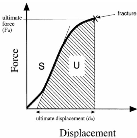
**Fig. 9.** A force displacement curve resulting from a biomechanical test of a specimen. The height of the curve (ultimate force) represents strength, area under curve is the work of failure (U), the maximum slope of the curve is stiffness (S).
