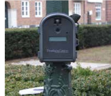
Figure 11. The timelapse camera mounted on a lamppost.
