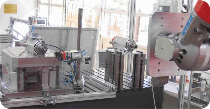
**Figure 2.5** Prototype machining cell for evaluation of the effectiveness of the proposed micro manipulator, which is seen to the left. The machining spindle to the right is rigidly attached to the base, and is utilized for milling experiments without compensation.
