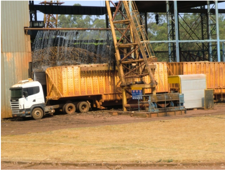
Figure 3.7. At the mill, the truck unloads and the cane is washed
