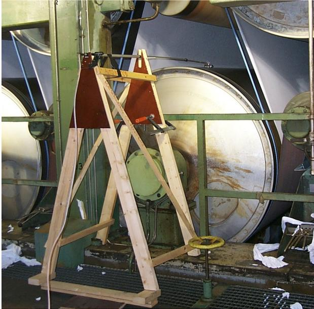
**Figure 5.6** Steam cylinder temperature measuring
