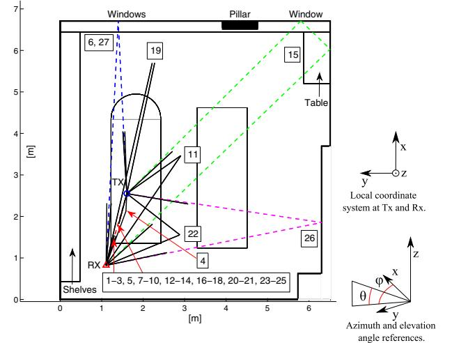
Fig. 3. Floorplan of the meeting room where the measurements took place with the Tx in one of 17 positions. The black lines are the azimuth estimates for the 27 strongest components in the LOS scenario.
