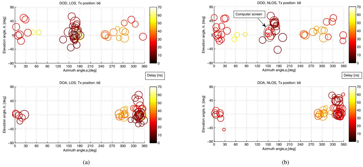
Fig. 5. Fig. 4. DOD and DOA for the (a) LOS and, (b) NLOS scenarios with the Tx in position b6.
