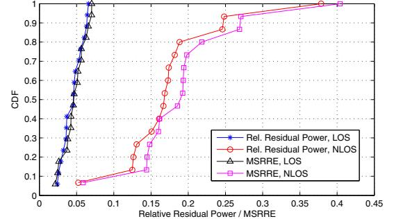
Fig. 1. CDFs of the relative residual power and the MSRRE for the different Tx positions in the LOS and NLOS scenarios.
