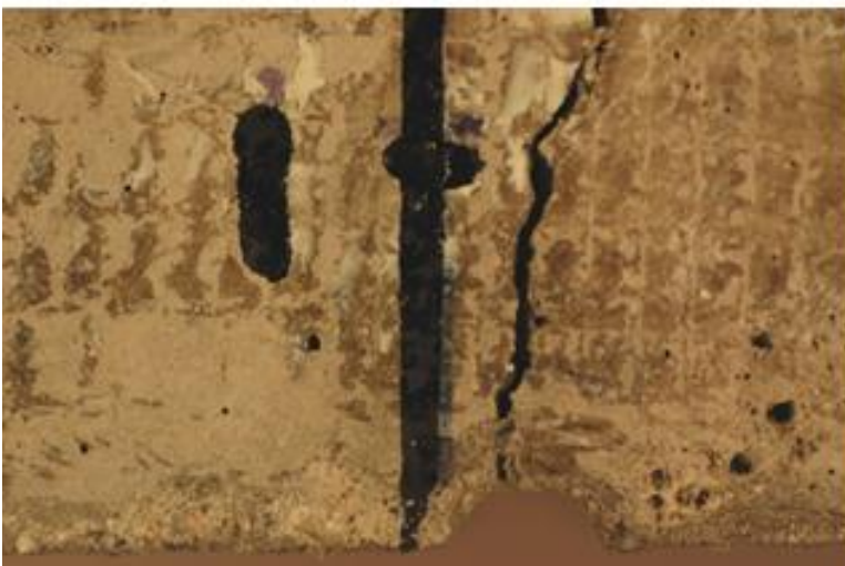
Figure 12.5: 0.4 mm crack after 28 month exposure to sea water. Concrete cover 55 mm.
