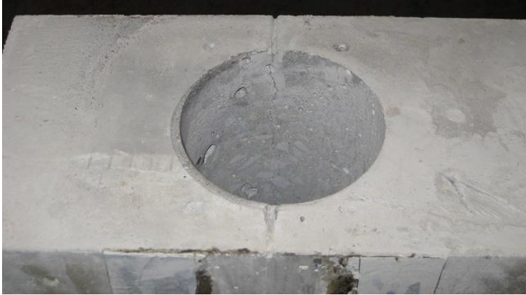
Figure 14.1: Example of a specimen after the core has been drilled out.
