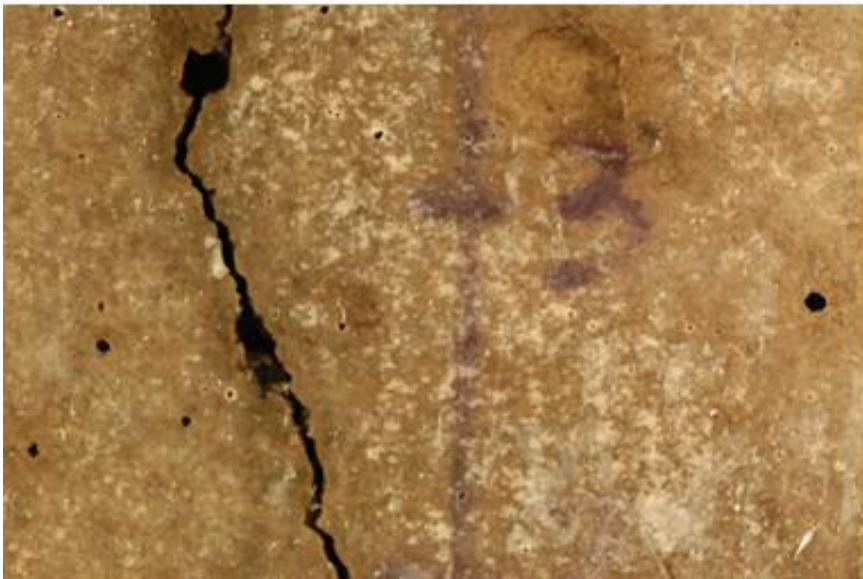
Figure A2.6: 0.4 mm crack width. Exposure to pure water. Upper: 75 mm cover. Lower: 55 mm cover.
