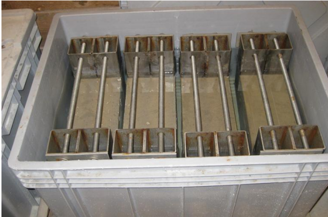
Figure 10.1: Water exposure type 1; permanently under water.
