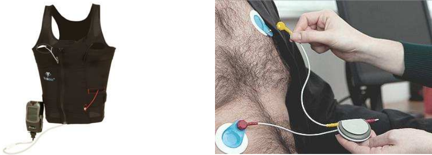
Figure 3.5 Vital signs sensor systems used in the DIAdvisor project; the VivoMetrics' LifeShirt system [VivoMetrics, 2012] (left), and the Sensium Life Pebble sensors by Toumaz [Toumaz, 2012] (right).
