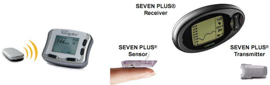
Figure 3.4 CGM systems used in the DIAdvisor project; the Abbott Freestyle CGM system, [Abbott Freestyle Navigator, 2015] (left), and the Dexcom Seven Plus CGM system [Dexcom Seven Plus, 2012] (right).
