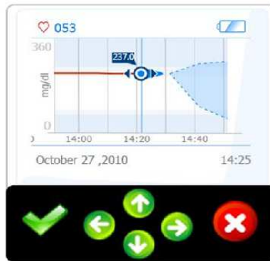
Figure 3.1 User Interface of the DIAdvisor system patient application implemented on the UMPC. On the screen, the user can follow the present and recent glucose values together with a projected future trajectory within specified uncertainty limits. Other vital signs, such as heart rate (see upper left screen corner), may also be possible to follow. User inputs, regarding, e.g., insulin and meal intake, are provided by a menu system controlled by the buttons at the bottom of the screen. Reproduced from [The DIAdvisor Consortium, 2012].
