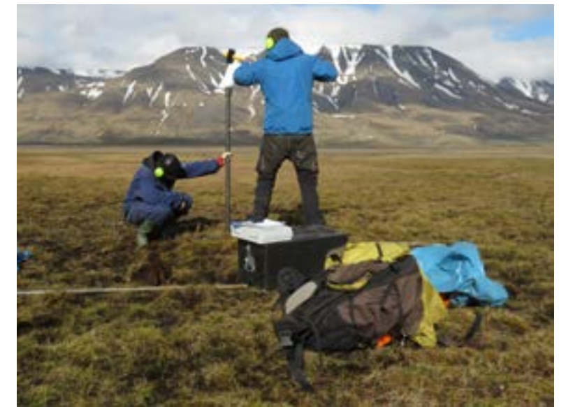
Figure 6. Field work in Adventdalen, Svalbard. The collection of soils is carried out by hammering a fixed volume steel tube into the frozen ground.
