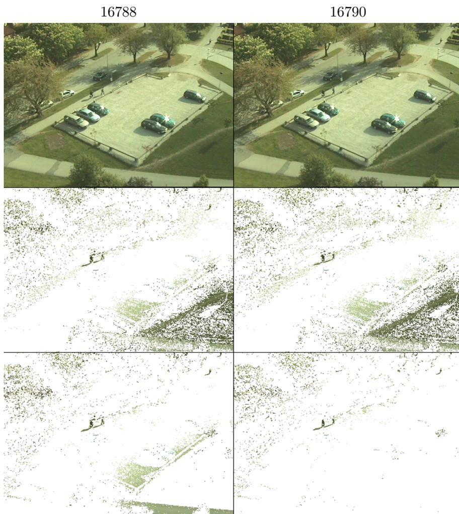
Figure 6: Results for a correctly detected illumination change using the segmentation algorithm in (Stauffer & Grimson, 1999). From top to bottom, frame number, original data, detected foreground with no intervention, and with altered background model and increased forgetting factor. The difference in segmentation prior to the detection is due to previous compensations for illumination changes. Note that the two pedestrians remain after altering the background model.
