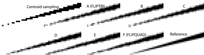
Figure 4: A thin polygon rendered using the sampling schemes, A through F, from Figure 3. The upper left polygon uses a single sample point per pixel while the reference polygon is supersampled with 1024 jittered grid sample points and uses a 4 \times 4 pixel Mitchell-Netravali reconstruction filter.
