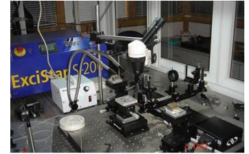
Figure 5.3. The FBG fabrication system at Zhejiang University.
