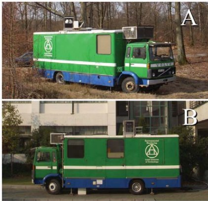
Figure 1. The lidar system at (A) the Swedish and (B) Chinese site. The transmitting dome is on both pictures currently mounted.
