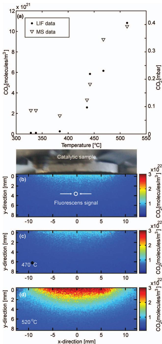
FIG. 5. (a) The CO<sub>2</sub> concentration 3.5 mm below the Rh(553) surface, (b) the position of the catalytic sample and where the fluorescence signal was averaged, (c) an estimate of the CO<sub>2</sub> concentration below the catalyst at 470 °C and (d) an estimate of the CO<sub>2</sub> concentration below the catalyst at 520 °C. The gas composition was 60 mbar of CO and 40 mbar of O<sub>2</sub>.
