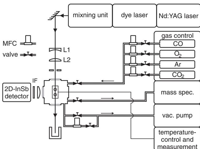
FIG. 1. Schematic of the experimental set up.
