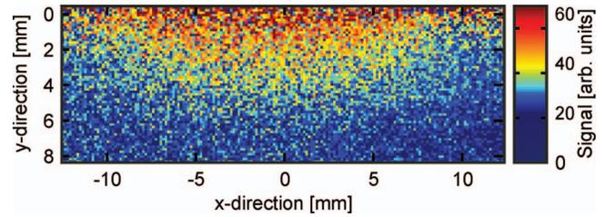
FIG. 4. Single-shot image (15  $\mu$ s exposure time) of the CO<sub>2</sub> distribution underneath a Rh(553) catalyst at a total pressure of 100 mbar with 60 mbar of CO and 40 mbar of O<sub>2</sub>.
