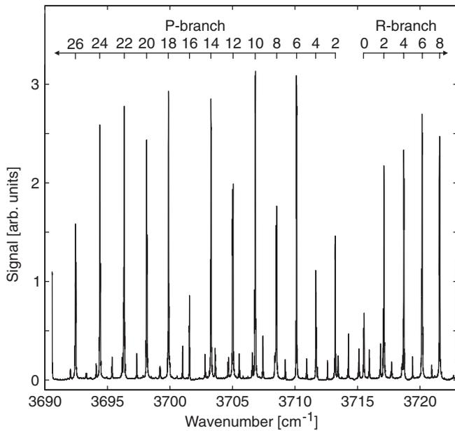
FIG. 3. CO<sub>2</sub> spectrum where the lines for the (00<sup>0</sup>0) → (10<sup>0</sup>01) transition are assigned. The smaller peaks are overtones and are not relevant to this work. P(12) was used for the fluorescence measurements.
