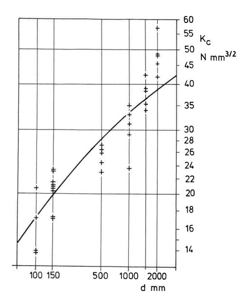
Fig. 1  $K_{\rm C}$  according to the Bologna tests as a function of the beam depth. The curve shows a theoretical relation for E = 24.6 GPa,  $G_{\rm F}$  = 160 N/m,  $f_{\rm t}$  = 2.1 MPa according to /3/.
