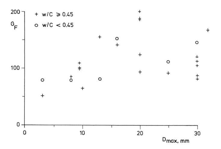
Fig. 2 Variation of  $G_F$  with maximum aggregate size and water/cement-ratio for standard beams according to the draft recommendations.
