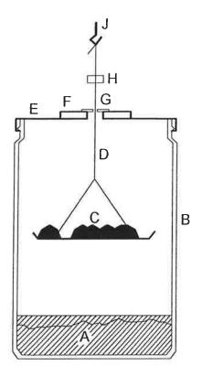
Figure 1. Drawing of the jar used in the measurements of sorption isotherms. A: saturated salt solution; B: glass jar; C: material to be investigated; D: wire; E: lid; F: metal plate; G: transparent washer; H: stop; J: hook on balance for under-weighing.
