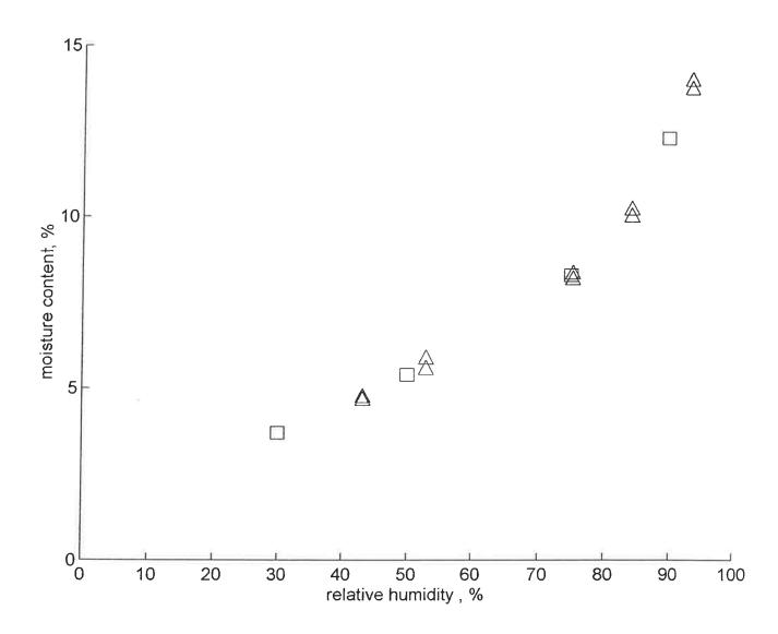
Figure 2. The result from a measurement of the sorption isotherm of cotton wool by the present method (triangles) and by Urquhart and Williams (squares). All measurements were made at 25°C.
