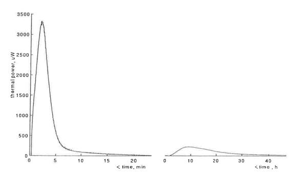
Results from an isothermal microcalorimetric measurement of the reaction between 80 mg cement (Cementa SRPC) and 40 mg water [1]. Note the different time scales of the two diagrams - the heat evolved in the second main peak is much larger than the heat of the early peak.
