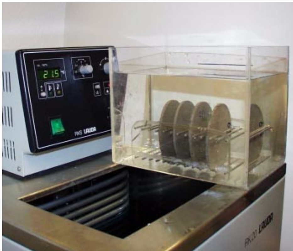
Figure 7.1.1: Cryostat, salt solution container and frame holding the specimens.
