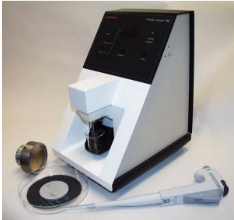
Fig 5.2.1: Grinding tool (far left), petri dish with abrasive cloth and specimen, pipette and potentiometric titration apparatus.
