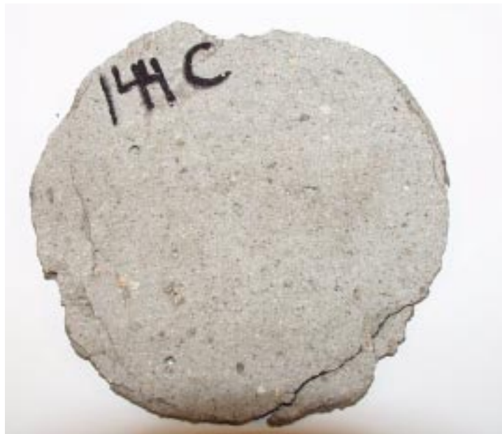
Figure 7.1.33: Cracks in thin specimen (appr. 2 mm). w/c ratio 0.40. Temperature -10^{\circ}\text{C} , outer concentration 14.4% NaCl, inner concentration 0%.
