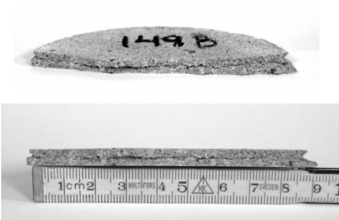
Figure 7.1.31: Crack in the center of w/c ratio 0.65 specimen stored in 3% NaCl solution for 19 days prior to test at -10°C, bath salt concentration 14.4%. (Two views)
