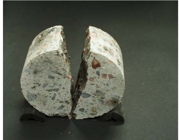
Figure 3.4 - The split specimen [4].
