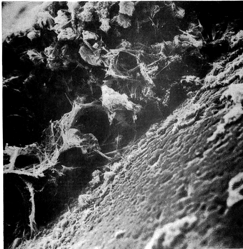
Fig 64: Scanning electrone microscope picture of cement mortar. 1:4. W_o/c = 0,54 . Porous interface paste - grain of aggregate. The grain to the right. Photo: Inst of Zoology. Univ of Lund.
