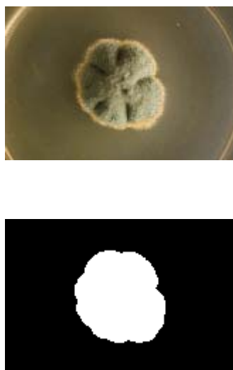
Figure 1. Colony surface area determination by image analysis program (MATLAB Image Processing Toolbox).
