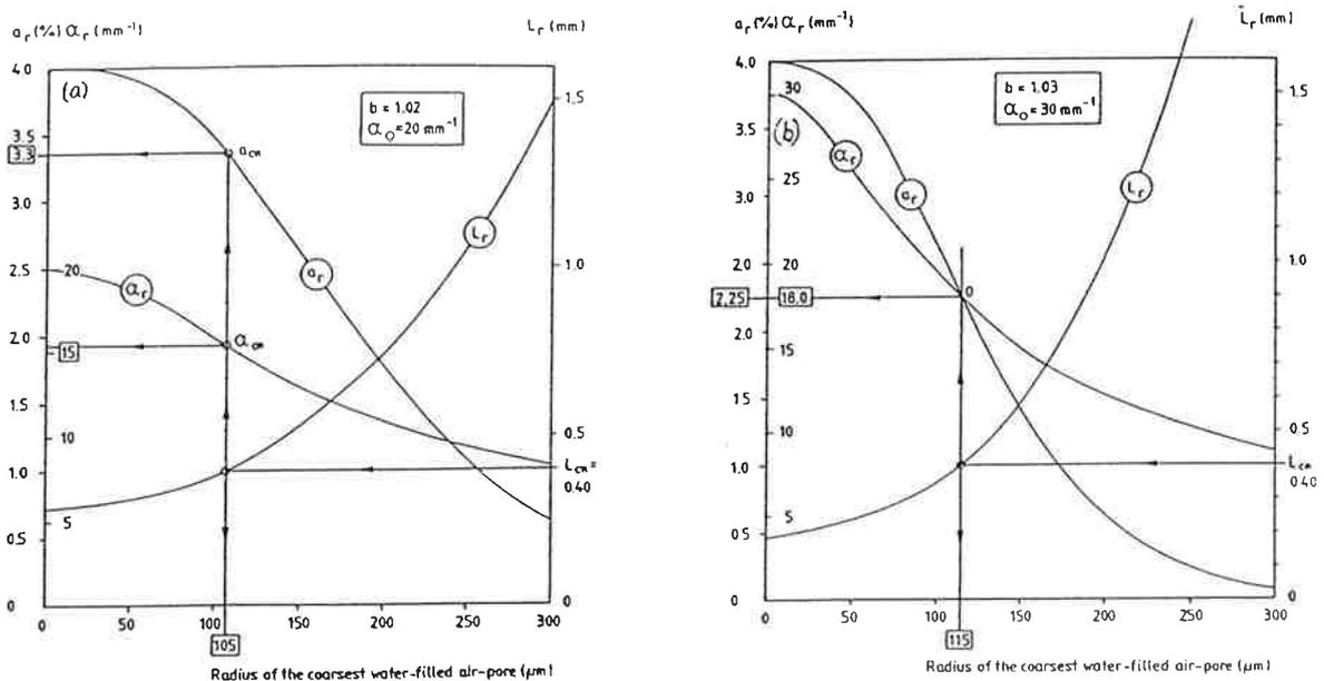
Fig. 3. Example of a calculation of the critical water absorption in the air-pore system.
