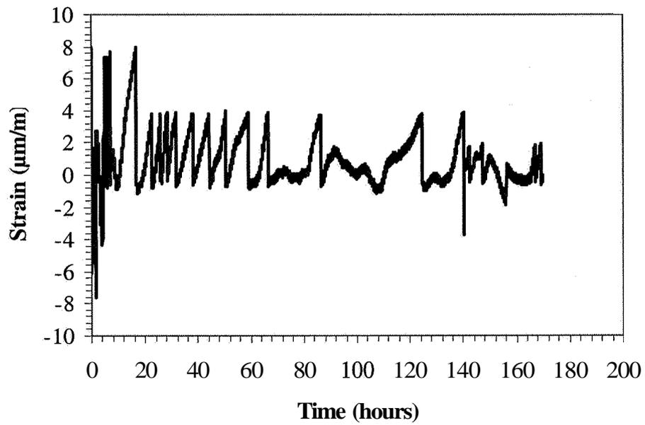
Figure 6. Restrained shrinkage W/C = 0,35
