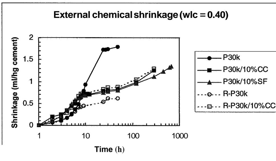
Fig 5 External chemical shrinkage versus time curves for P30k cement without (until 48 h) with 10% replacement of calcium carbonate (until 288 h) and silica fume (until 672 h) for  $w/s = 0.40$ . The legend R- means that the sample was rotated.
