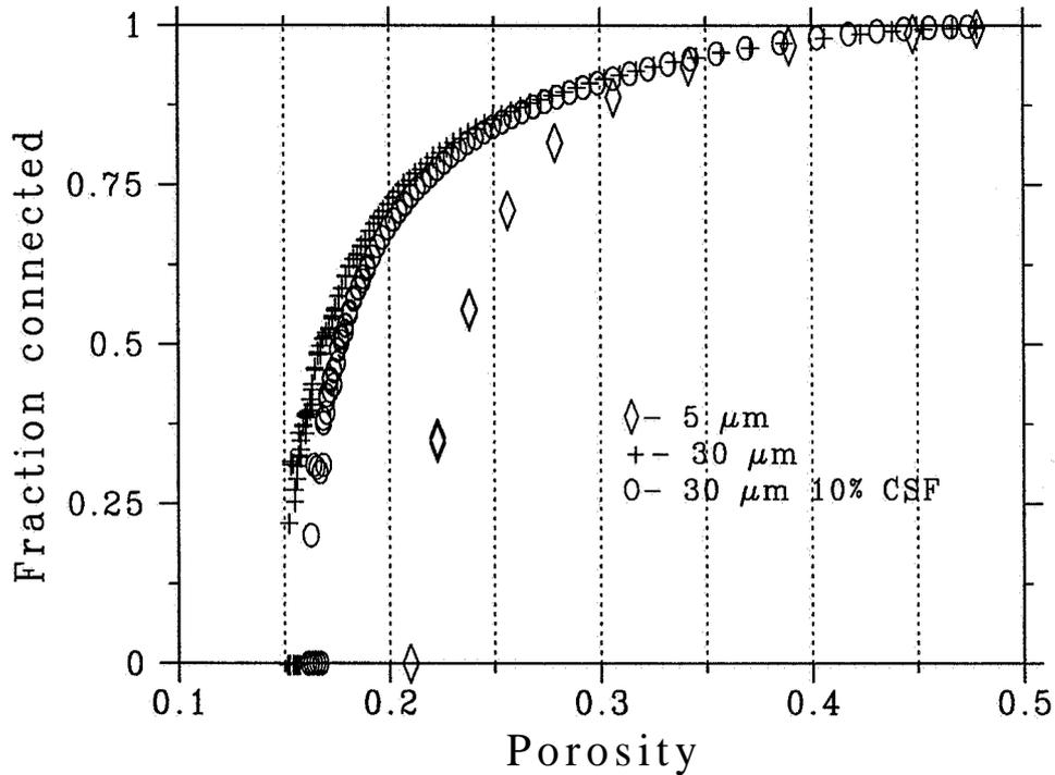
Fig. 1: Fraction connected porosity vs. total porosity for  $w/c=0.3$  cement pastes of varying cement PSD and silica fume content. System size is  $200 \times 200 \times 200$  ( $0.5 \mu\text{m}/\text{pixel}$ ).
