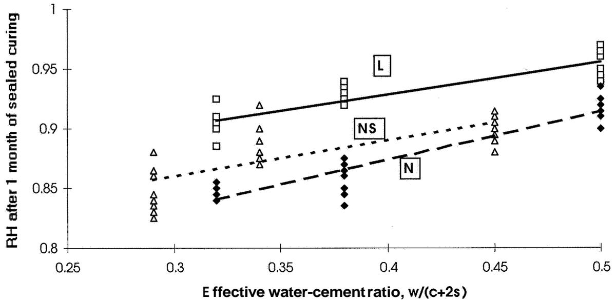
□ Lowalkali cement L ◆ Normal-alkali cement N ▲ Normal-alkalicement + 5% silica fume, NS
