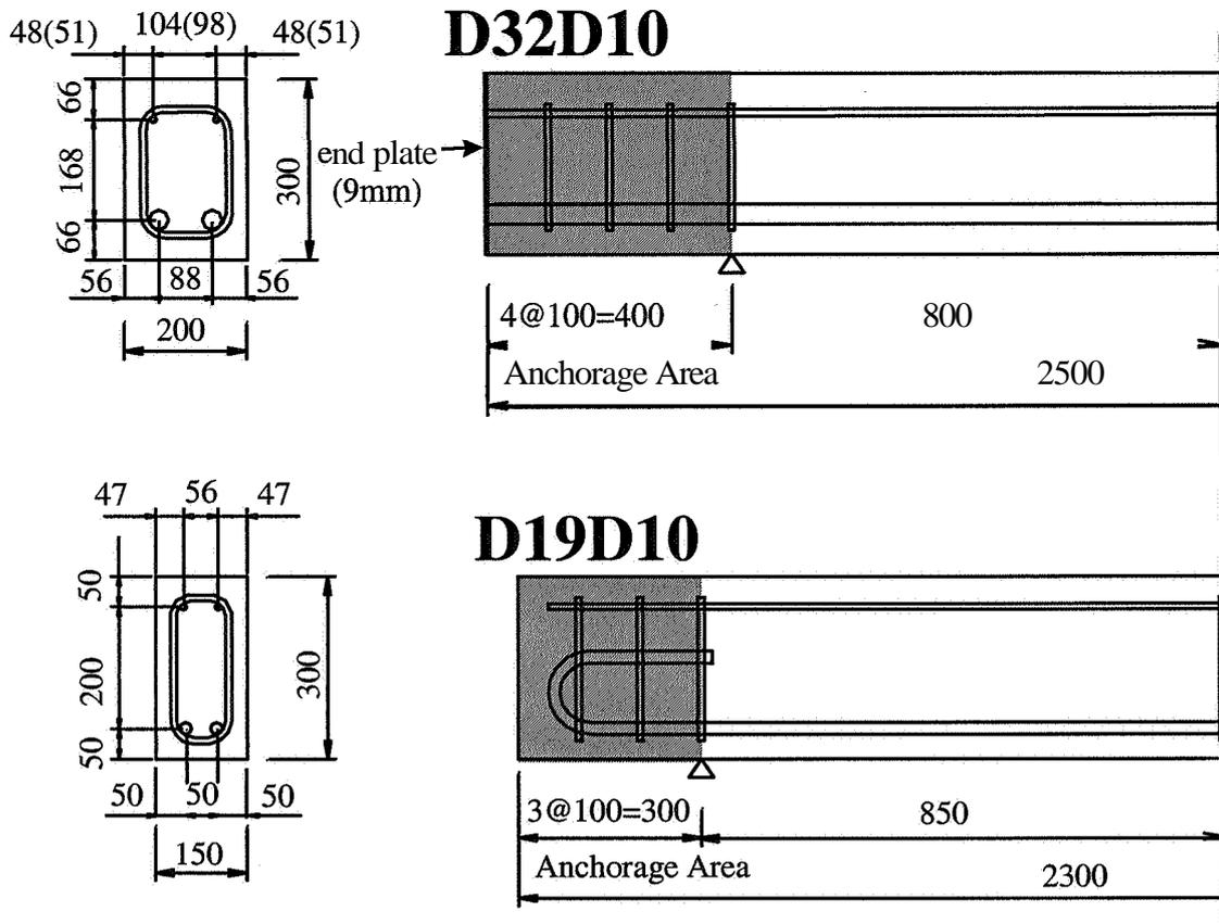
Fig. 1. Dimensions and configuration of steel bars of beam specimen.
