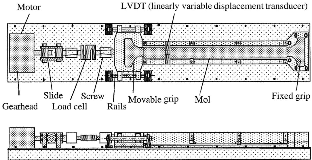
Figure 1. Restrained shrinkage apparatus
