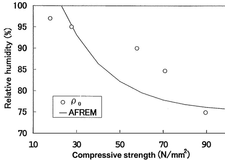
Fig. 13 Relation between compressive strength and relative humidity
