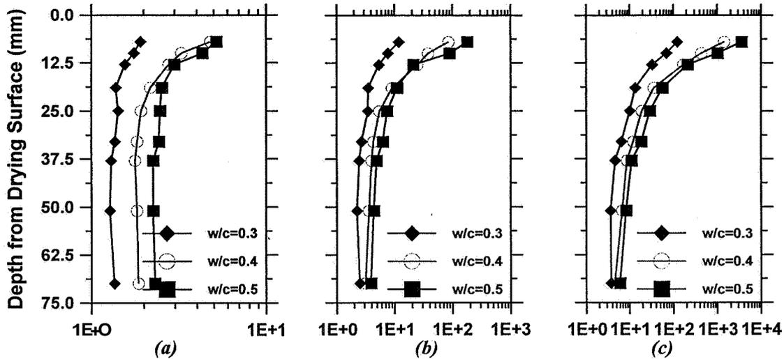
**Figure 9: Normalized Bulk Resistance Profiles for the Mixes Studied in this Investigation (a) 3 Days, (b) 28 Days, and (c) 98 Days**
