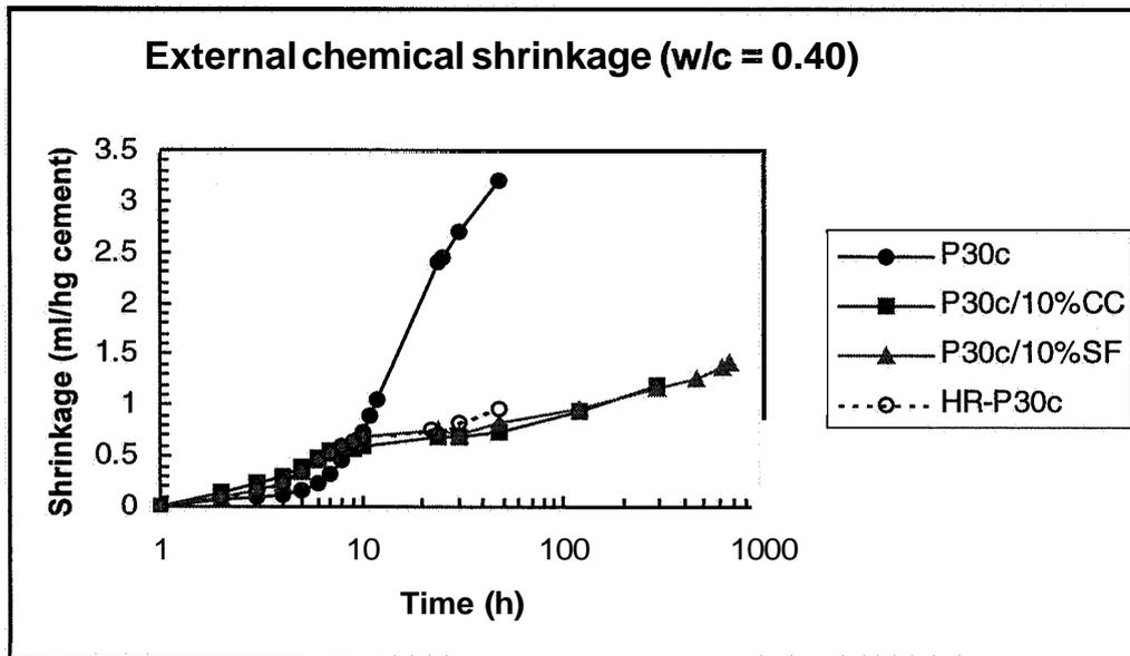
Fig 7 External chemical shrinkage versus time curves for P30c cement without (until 48 h) with 10% replacement of calcium carbonate (until 288 h) and silica fume (until 672 h) for  $w/s = 0.40$ . The legend HR- means that the sample was rotated by hand.
