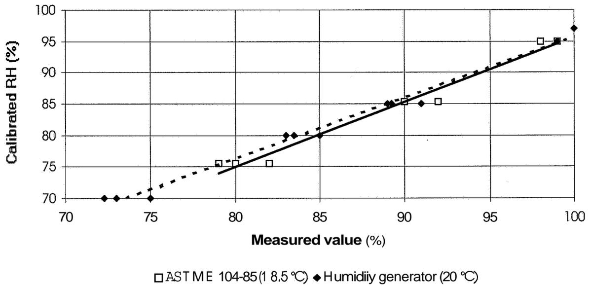
Fig. 14. RH calibrated according to ASTM E 104-85 (18.5 °C), [18], and according to humidity generator (20 °C).
