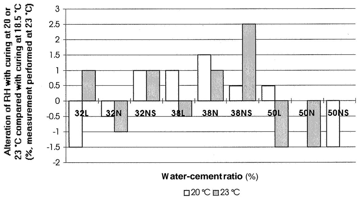
Fig. 5. Alteration of RH with curing at 20.5 °C and 23 °C compared with curing at 18.5 °C (measurement performed at 23 °C). L= low-alkali, N = normal-alkali, S = 5% silica fume, 32= w/c (%).
