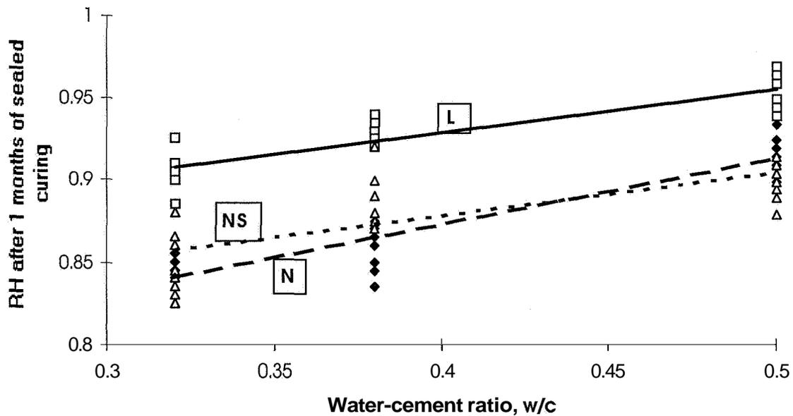
□ Low-alkali cement L ◆ Normal-alkali cement, N ▲ Normal-alkali cement + 5% silica fume, NS
