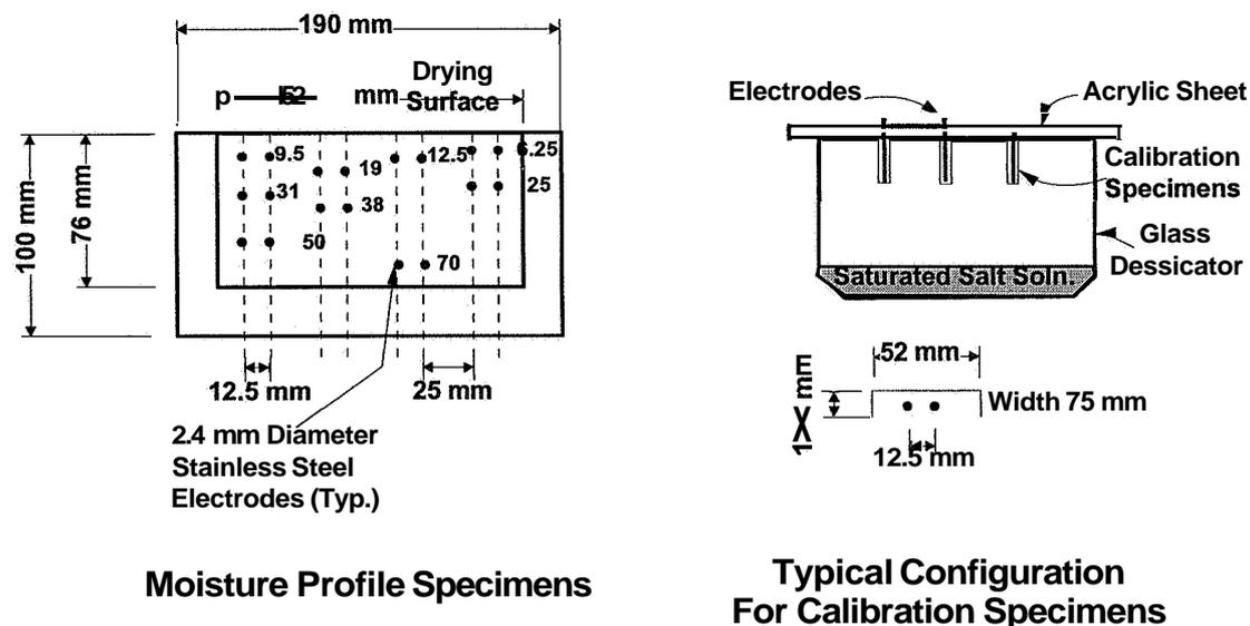
Figure 1: Specimen Geometry
