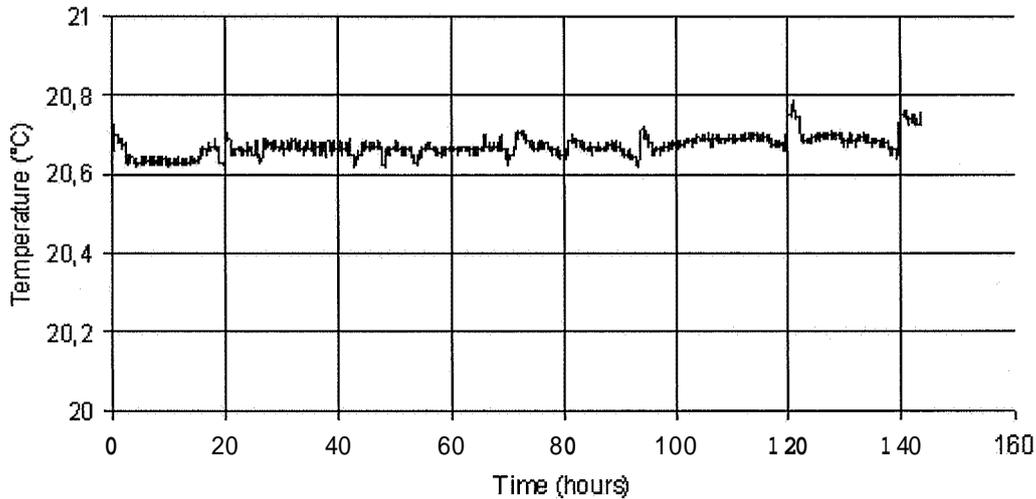
Fig. 10. Example of evolution of temperature in the surrounding water of the sample in the volumetric test.
