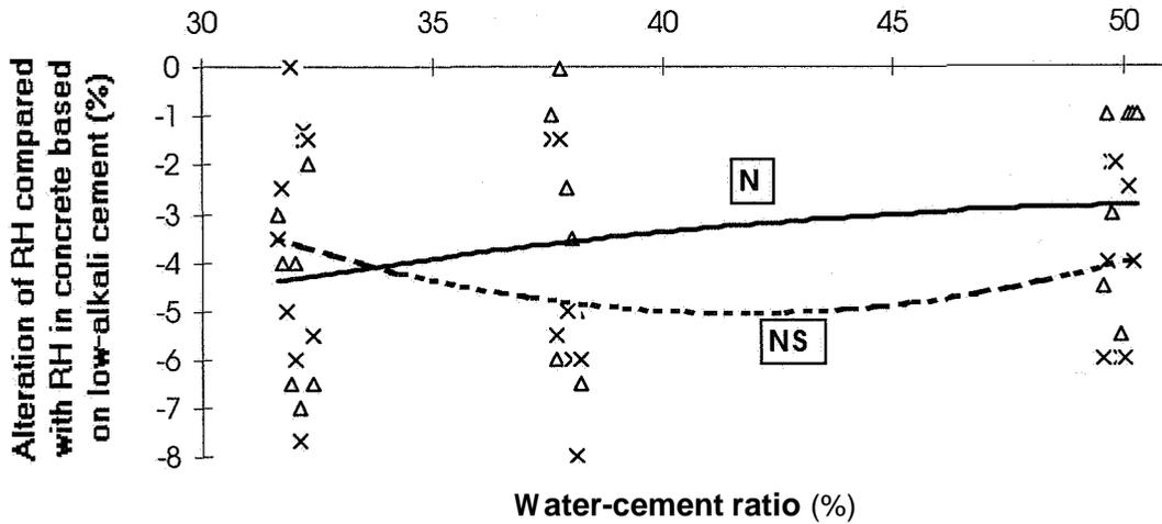
a N = Normal-alkali cement x NS = Normal-alkali cement + 5% silica fume
