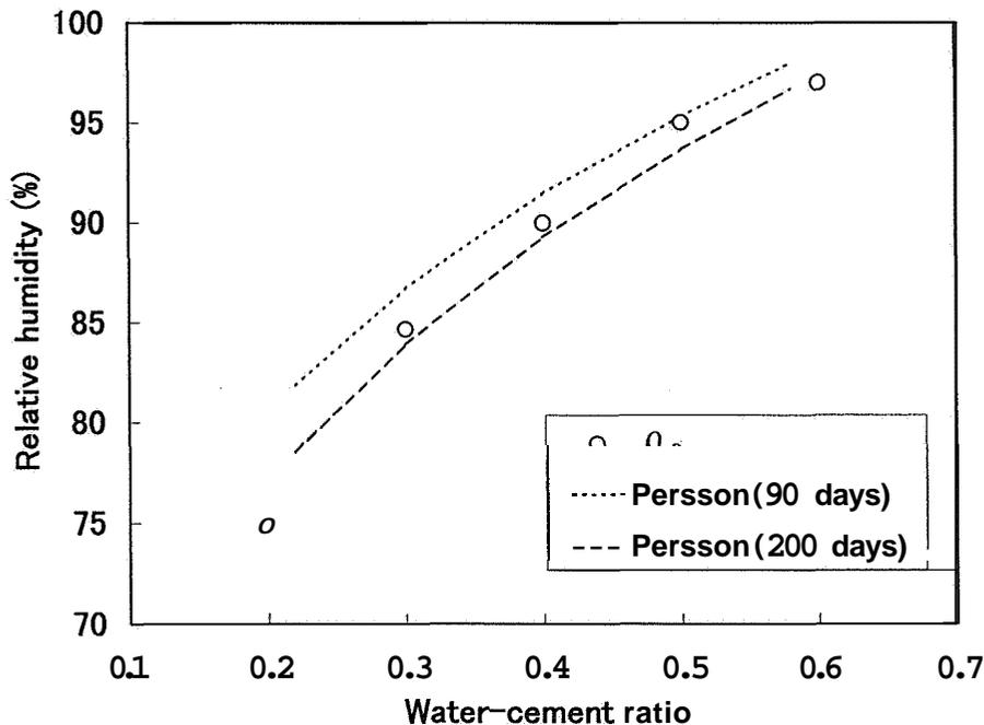
Fig.12 Relation between water-cement ratio and relative humidity
