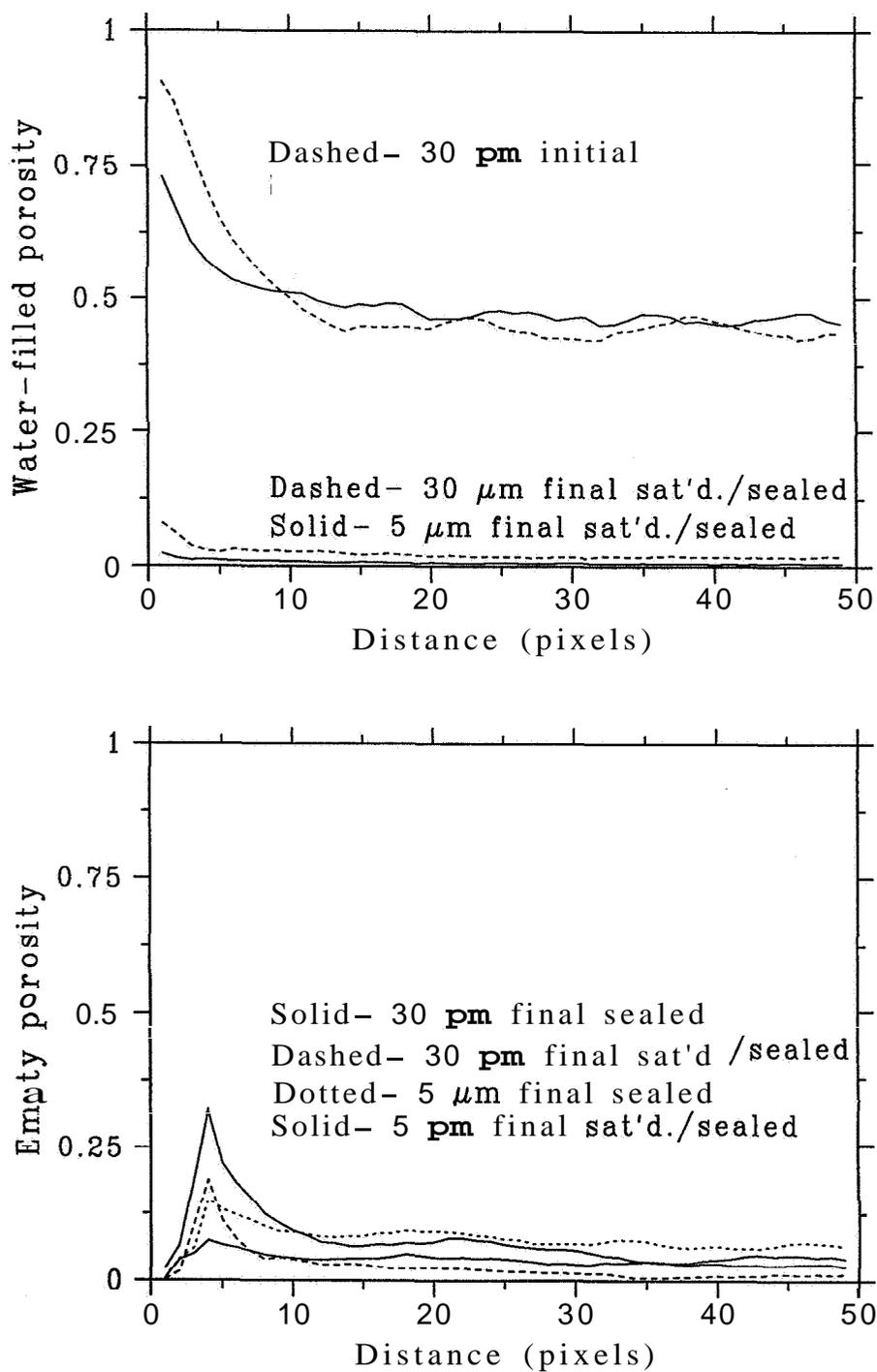
Fig. 3: Water-filled (upper) and empty (lower) porosity volume fractions vs. distance from aggregate,  $w/c=0.3$ . Final curves for empty porosity are for hydration under sealed or saturated/sealed curing conditions.
