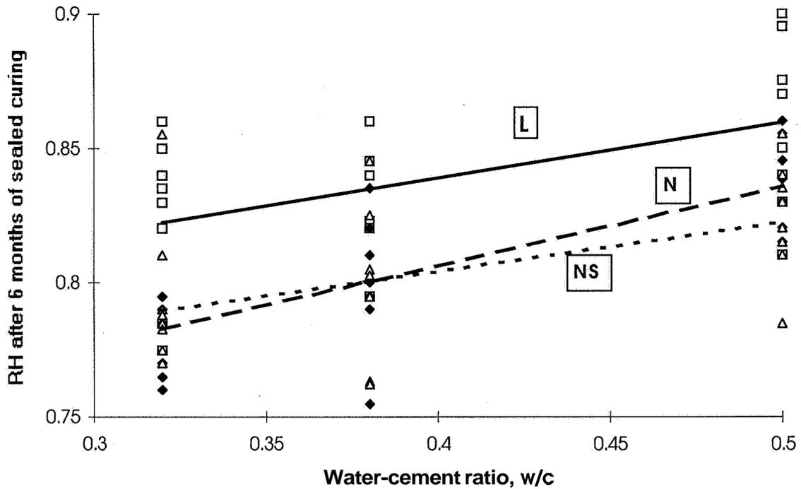
Fig. 20. RH versus w/c, 6 months' age. L= low-alkali, N = normal-alkali, S = 5% silica fume, 32= w/c (%).
