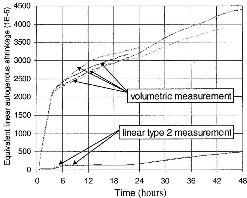
Fig. 2. Comparison of volumetric and linear results.
