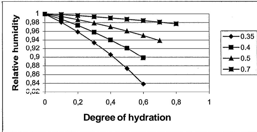
Fig. 4. Self-desiccation at different W/C-ratio.
