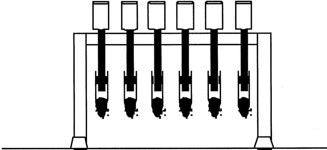
Fig. 2. During the measurement of moisture the device was entered into the pipe and tightened towards the inner face of the pipe by an expanding rubber ring,
