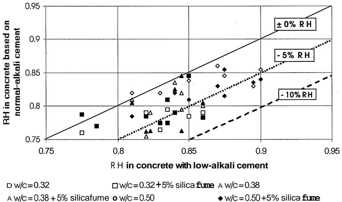
Fig. 18. Influence of cement type and silica fume on RH versus RH compared with RH in concrete based on low-alkali cement. Six months' age.
