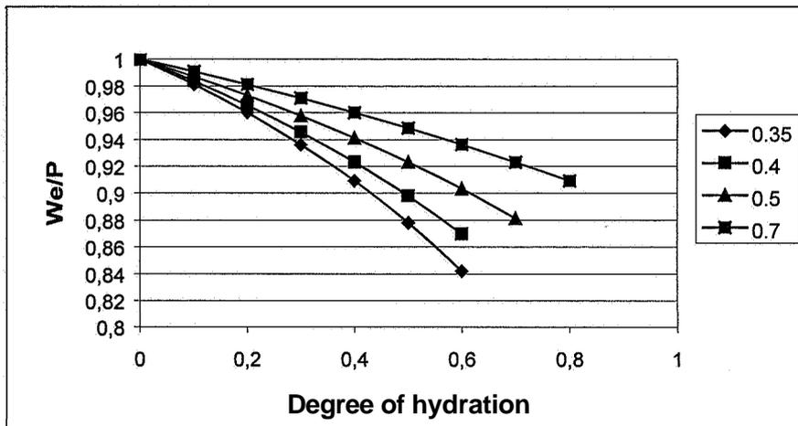
Fig. 1. The degree of saturation at different W/C-ratios.
