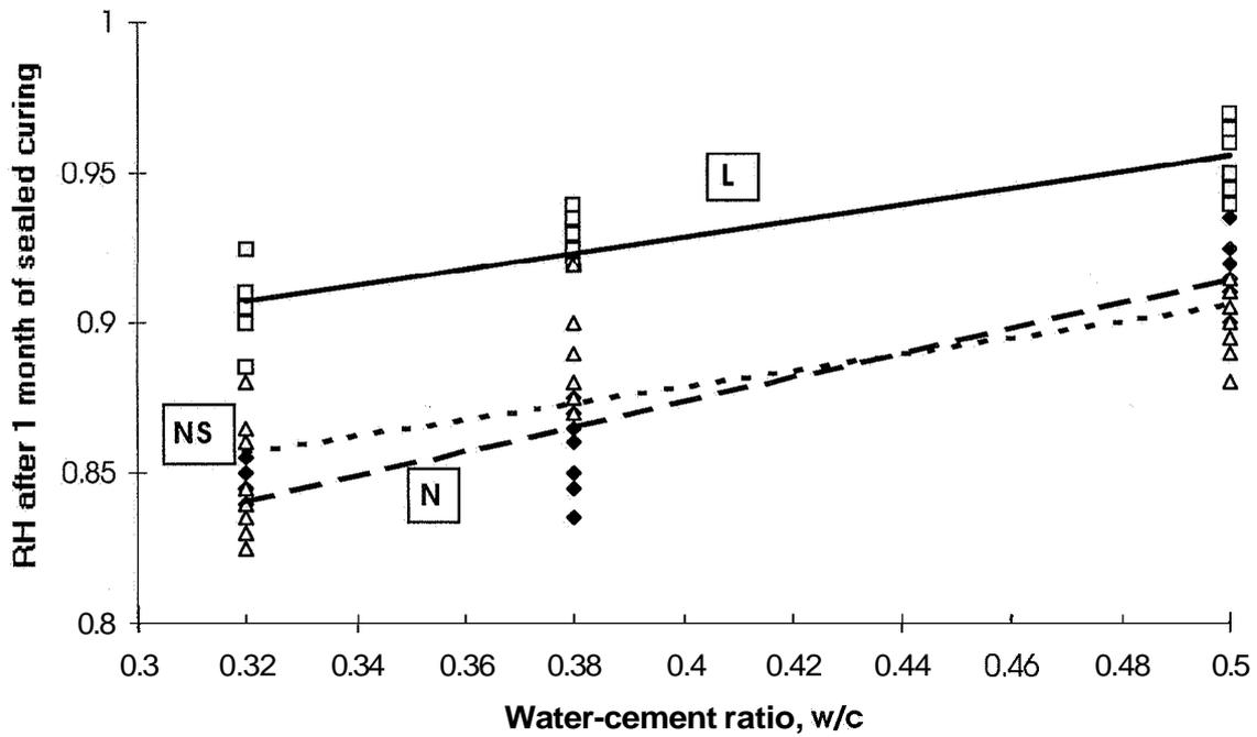
Fig. 19. RH versus w/c, 1 month's age. L= low-alkali, N = normal-alkali, S = 5% silica fume, 32= w/c (%).
