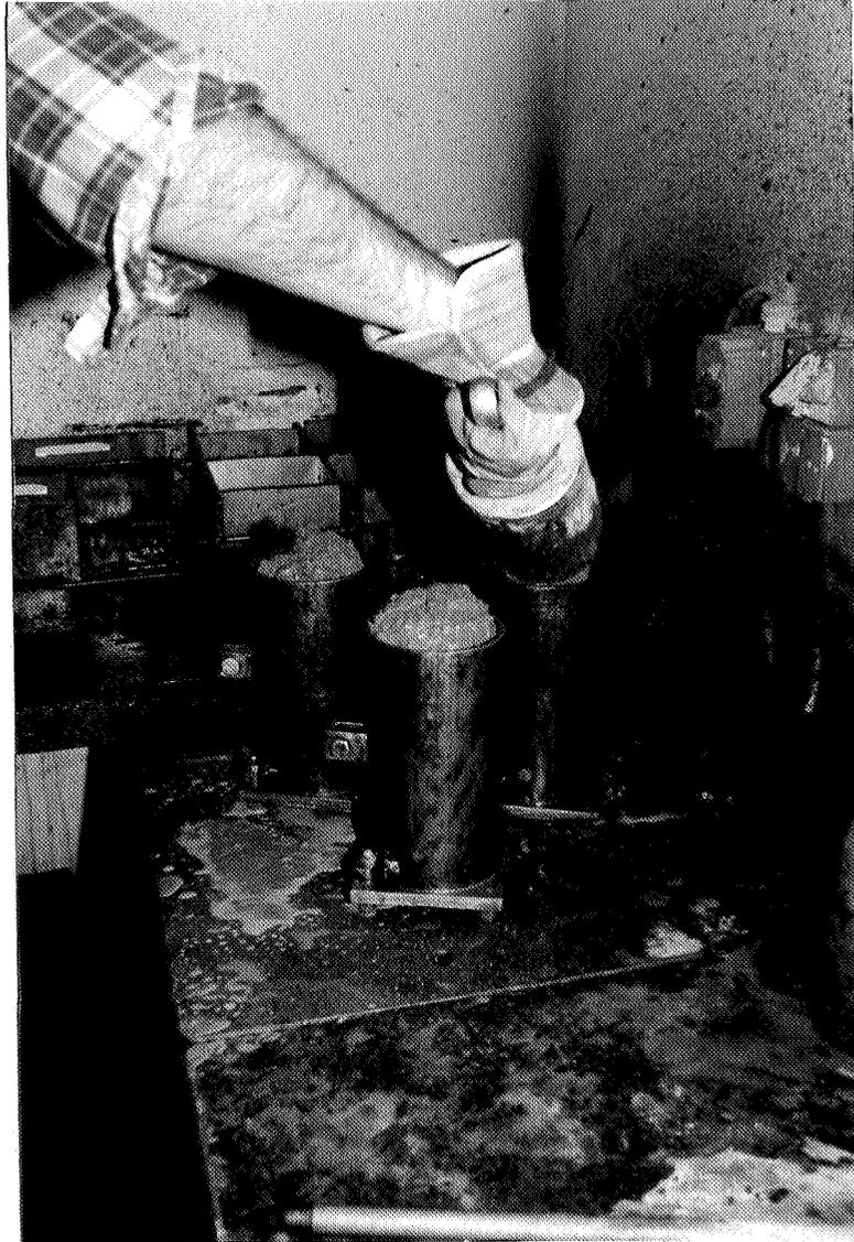
Fig. 5. Standard cylinders were fabricated at the concrete factory, i.e. sample of concrete was taken directly from the transport of concrete [6].
