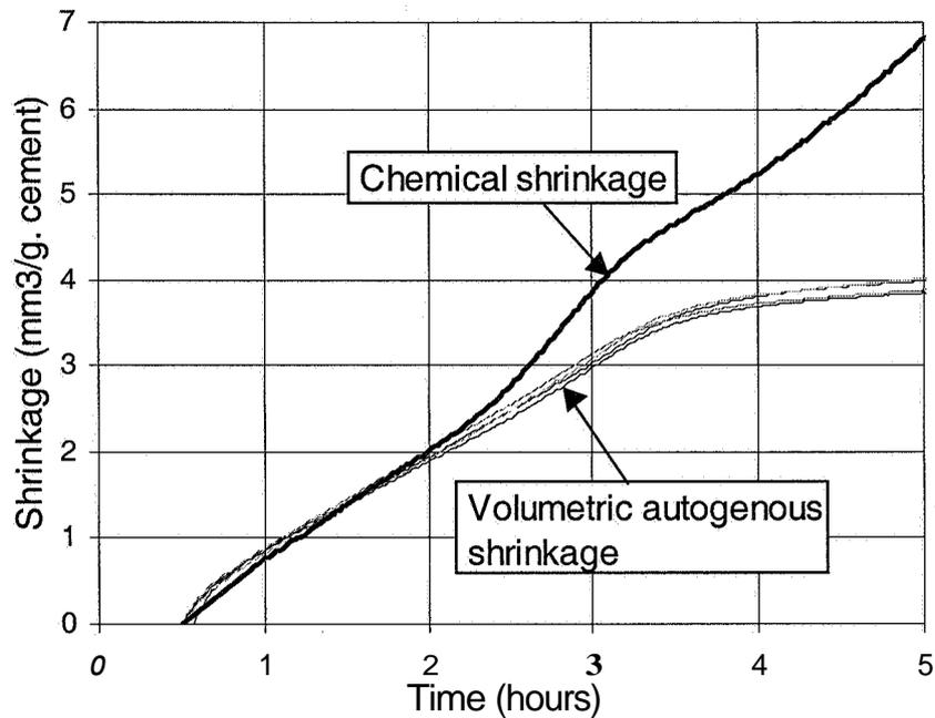
Fig. 4. Volumetric autogenous shrinkage vs chemical shrinkage.
