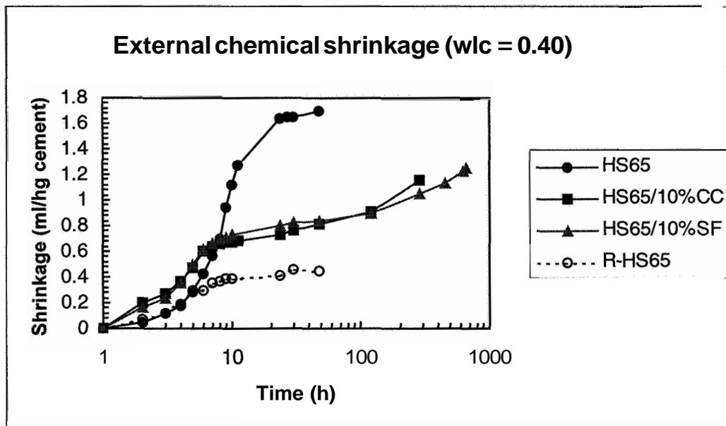
Fig 9 External chemical shrinkage versus time curves for HS65 cement without (until 48 h) with 10% replacement of calcium carbonate (until 288 h) and silica fume (until 672 h) for  $w/s = 0.40$ . The legend R- means that the sample was rotated.
