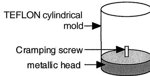
Fig. 1. Testing equipment for linear vertical measurement.
