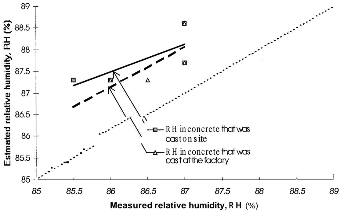
Fig. 8. RH estimated according to equation (1) versus RH measured in field tests [6].
