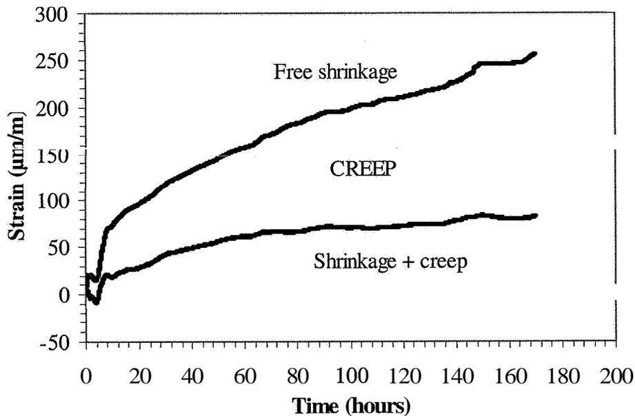
Figure 2. Cumulative curve of strains versus free shrinkage
