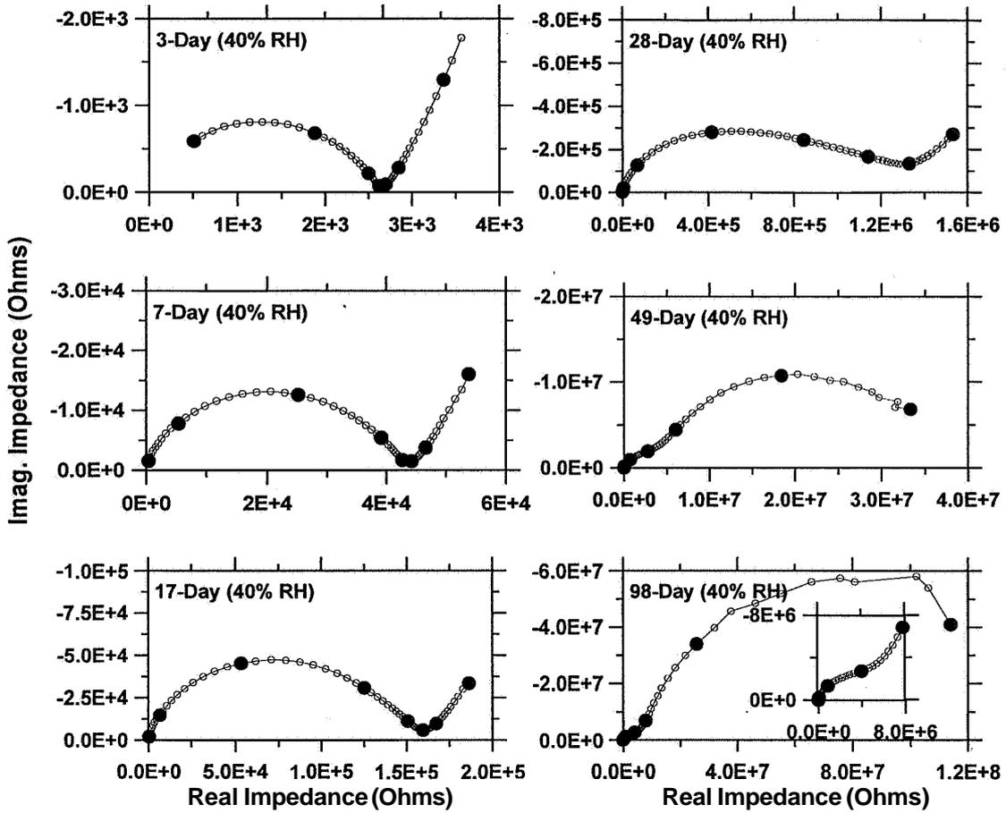
Figure 5: The Measured Nyquist Response for Paste as Drying Occurs for a  $w/c = 0.5$  Mixture in a 40% Environment (Note: Solid Circles Correspond with Decade Frequencies While Open Circles Correspond to Individual Measurements)
