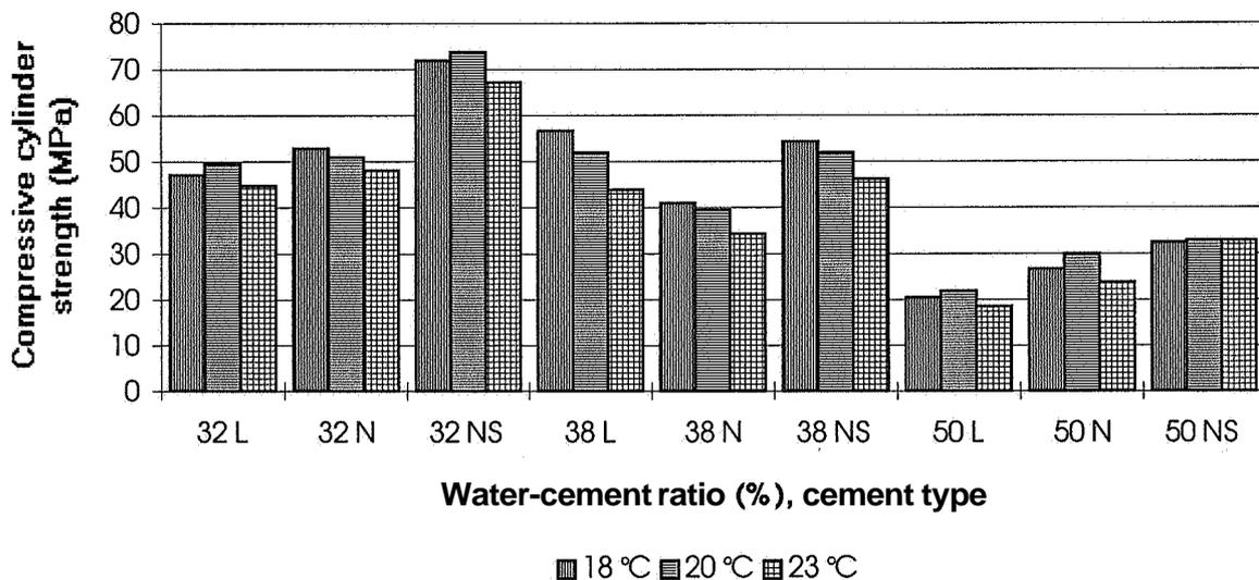
Figure 2. Strength versus w/c and type of the concretes. L= low-alkali cement, N = normal-alkali cement, NS = N+ 5% silica fume, 32= w/c (%).
