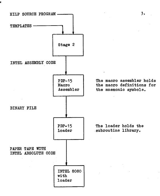
fig 1. From HILP 80 source to loaded INTEL 8080.
