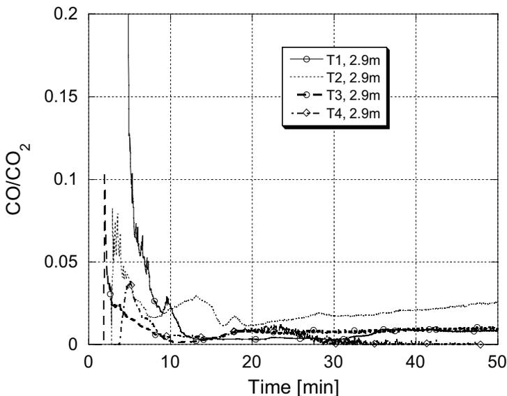
Figure 6.3 CO/CO<sub>2</sub>-ratio as function of time for the Runehamar tests. The gas analyses were performed at 458 m from the centre of the fire, 2.9 m above the road surface.
