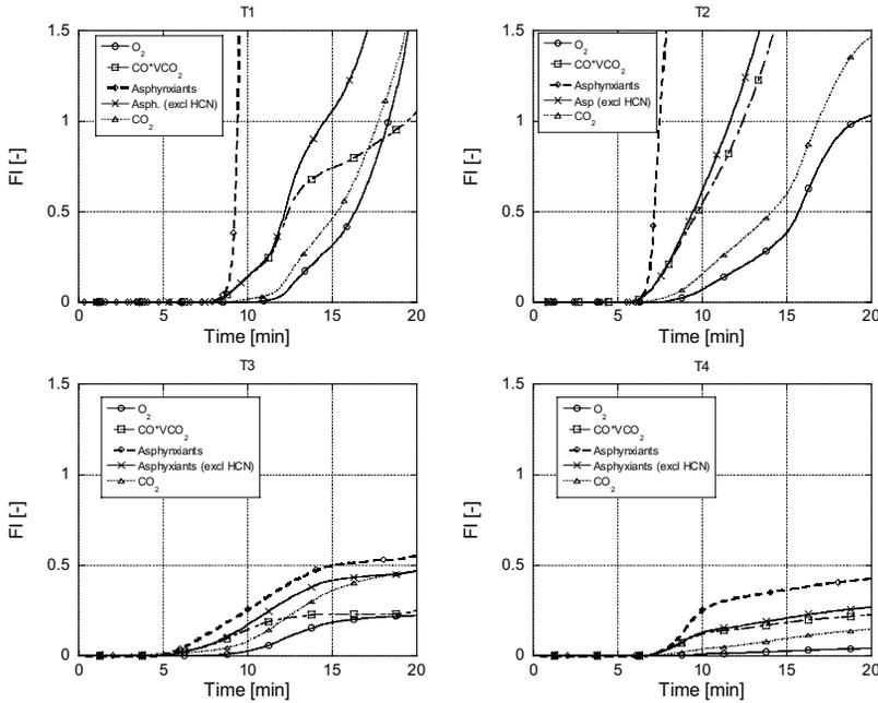
Figure 6.5 Fraction of an incapacitating dose for asphyxiant gases analysed during the four tests in the Runehamar tunnel.
