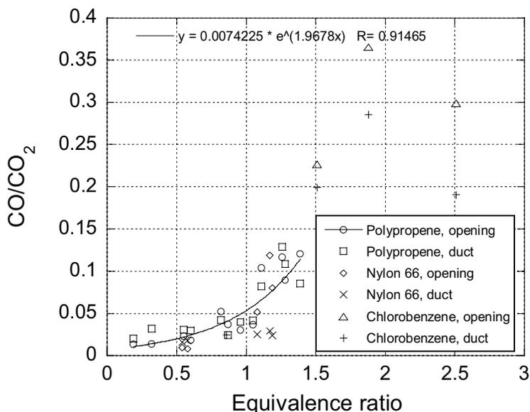
Figure 6.2 CO/CO<sub>2</sub>-ratio as function of equivalence ratio for polypropene, Nylon 66, and chlorobenzene. For all three materials, results are given for measurements in the opening of the enclosure and in the exhaust duct connected to the hood collecting the fire gases. An exponential curve fit is included for polypropene (opening).
