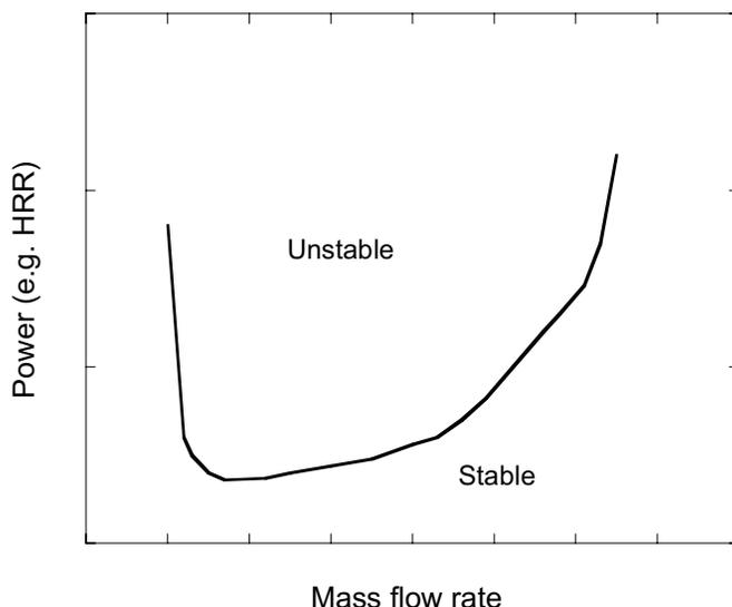
Figure 5.3 Example of stability limit (after Matveev [215]).
