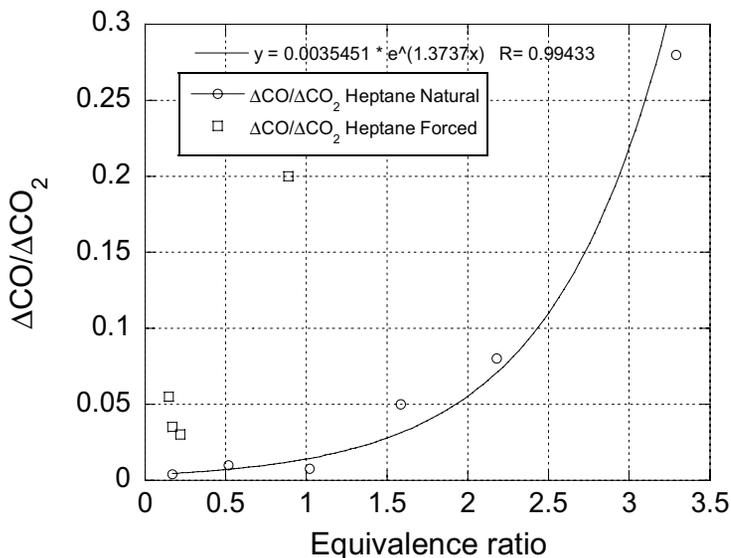
Figure 6.1  $\Delta\text{CO}/\Delta\text{CO}_2$ -ratio as function of equivalence ratio for heptane pool fires performed by Ingason [42, 43]. The results are given both for natural ventilation and for forced ventilation. Included for illustration is an exponential curve fit of the natural ventilation data. It is, however, based on only six data points.
