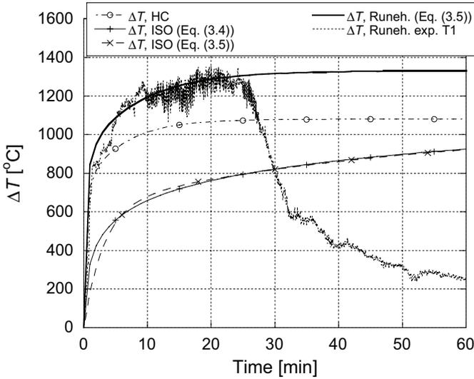
Figure 3.4 Comparison of different fire curves based on Eq (3.4) and Eq (3.5) with results from the results from the Runehamar tunnel.
