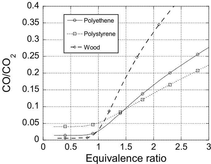
Figure 6.4 CO/CO<sub>2</sub> ratio for polyethene, polystyrene, and wood as a function of  $\phi$ , based on the work by Tewarson (Eq. (6.2)) [35].
