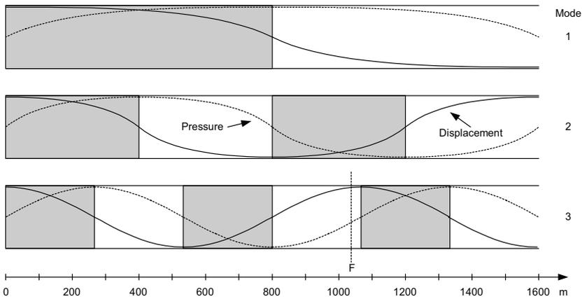
Figure 5.4 The figures represent the amplitude for the first three modes of oscillations in a tube (the top one is the fundamental). The length scale of the Runehamar tunnel is included for comparison. The vertical dashed line (F) represents the position of the centre of the fire during the tests in the Runehamar tunnel. The shadowed areas indicate regions favourable for instability for each mode.
