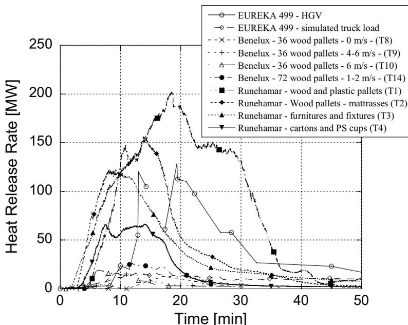
Figure 3.2 The time resolved HRR for the HG, trailer simulation tests from three different test series.
