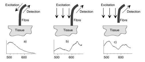
Fig. 21. Illustration of the influence of the measurement set-up to the detected fluorescence signal, from Eker<sup>112</sup>.
