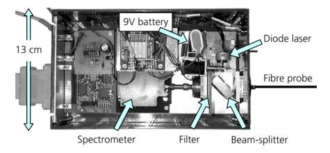
Fig. 22. Top view of the diode fluorosensor.
