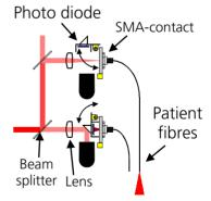
Fig. 27. Left: System overview (IPDT-I), from Paper III. 1) Treatment laser, 2) Light distribution unit, 3. Computer, 4. Treatment fibres. Inset left: top view of the light distribution unit. Right: Detail from the light distribution unit showing one patient fibres in treatment mode (top) and one fibre in detection mode with the photodiode measuring the light intensity at the fibre tip (bottom), from Paper VI.
