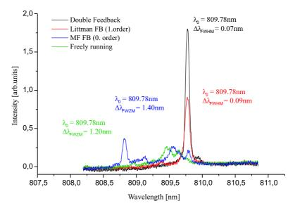
Fig. 3. Spectrum of the double and single feedback laser. Black spectrum: Double feedback applied; Red spectrum: Feedback from first order applied; Blue spectrum: Feedback from zeroth order applied; Green spectrum: Freely running laser.
