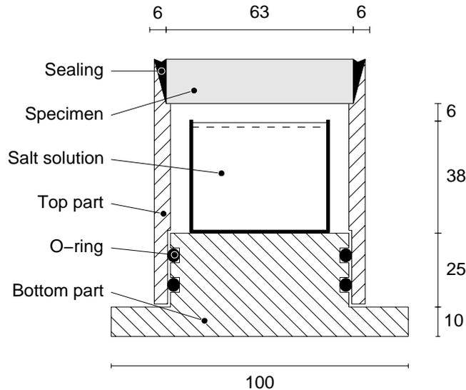
Figure 1– Schematic picture of the cup used. Different top parts have different heights of the bevelled part to fit specimens with different thickness.
