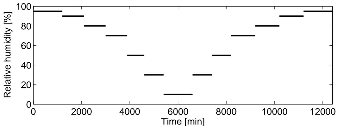
Figure 2 – Test cycle used in experiments. Measurements started and ended at 95% RH.
