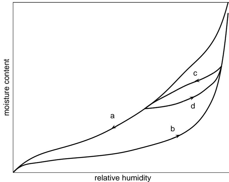
*Figure 1 – Example of a sorption isotherm, where **a** is a desorption isotherm, **b** an absorption isotherm, **c** a scanning curve from the absorption isotherm to the desorption isotherm and **d** a scanning curve from the desorption isotherm to the absorption isotherm.*
