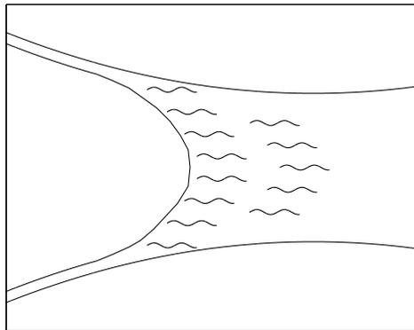
Figure 5.1: Schematic drawing of water meniscus formed in a pore.
