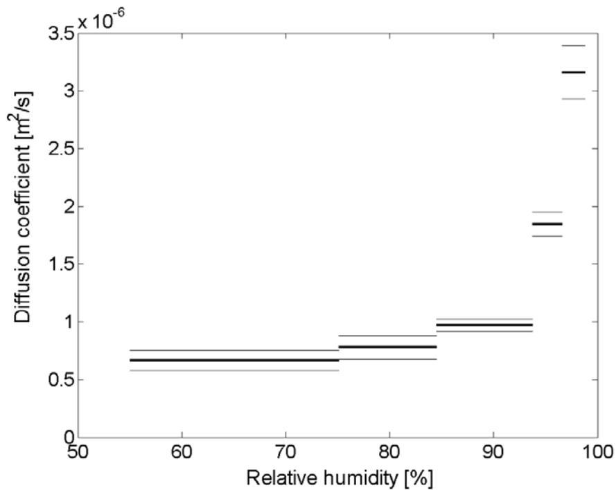
Figure 3 – Diffusion coefficient for SLC A. Thick line is the mean value in the shown interval. Thin lines indicate one standard deviation.
