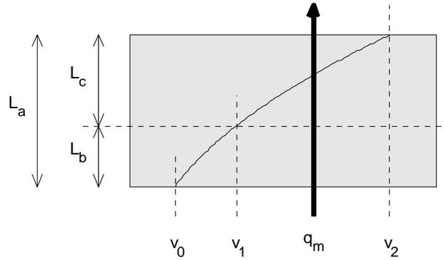
Figure 2 – A schematic drawing of a cup measurement made with a specimen of thickness  $L_a$  between vapour contents  $v_0$  and  $v_2$ . Also shown is the division of the specimen into two specimens of thickness  $L_b$  and  $L_c$  and how one will get the same flow as with the thicker specimen by making measurements in the interval  $v_0$  to  $v_1$  and  $v_1$  to  $v_2$ , respectively.
