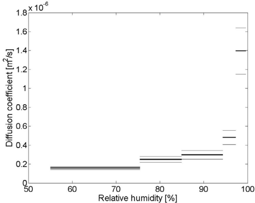
Figure 5 – Diffusion coefficient for SLC C. Thick line is the mean value in the shown interval. Thin lines indicate one standard deviation.
