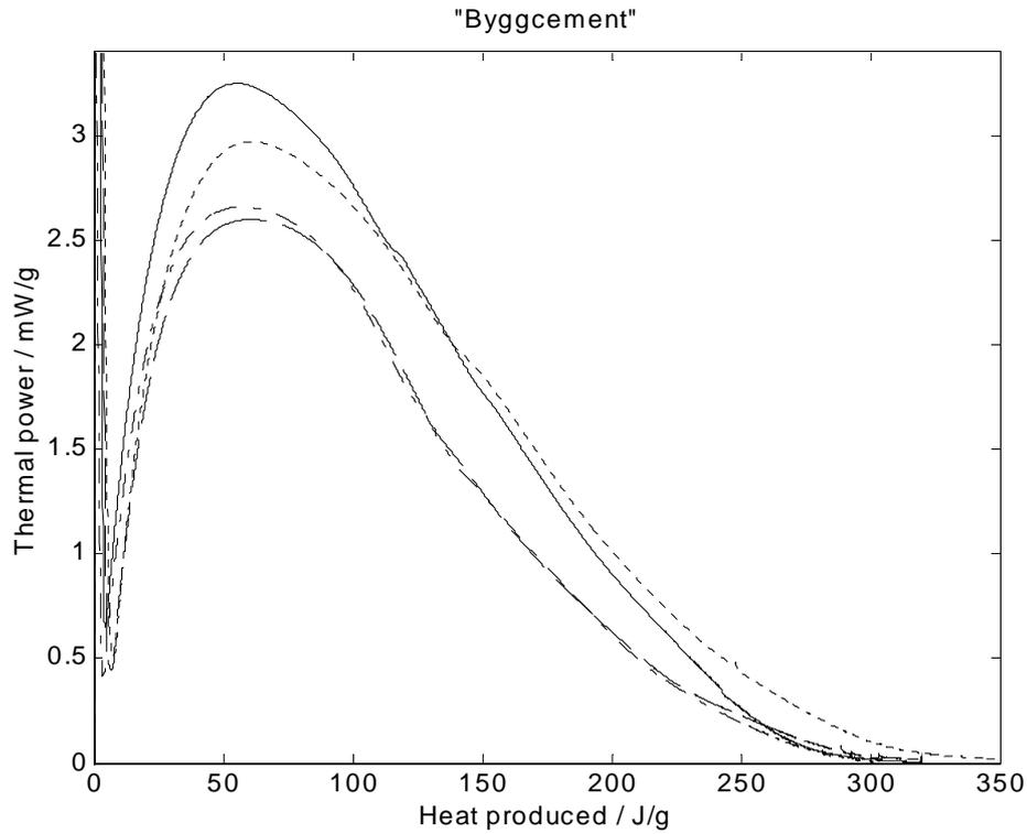
Figure 5 - Specific thermal power (watts per gram cement) as a function of produced heat (joules per gram cement) for the Portland limestone cement. Each curve is a mean of two measurements on samples from the same mix. The differences between two curves were never more than 0.1 mW/g. W/c=0.35 (solid), w/c=0.40 (dash-dotted), w/c=0.45 (dashed) and w/c=0.50 (dotted).
