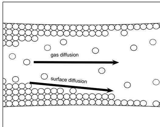
Figure 6.1: Schematic picture of diffusion in a pore, where molecules in random motion tend to move towards lower concentration.
