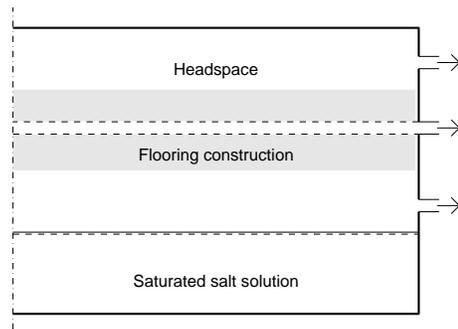
Figure 8.1: Schematic picture of test setup in [66].
