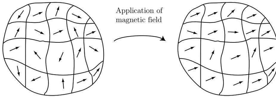
**Figure 2:** The alignment of domains when applying an external magnetic field. The configuration to the left shows the disordered domains in the absence of a magnetic field. When we apply an external magnetic field, the domains align themselves along the field (or rather: domains which are already aligned to the field grow on the expense of other domains). This alignment remains even after removing the external magnetic field.
