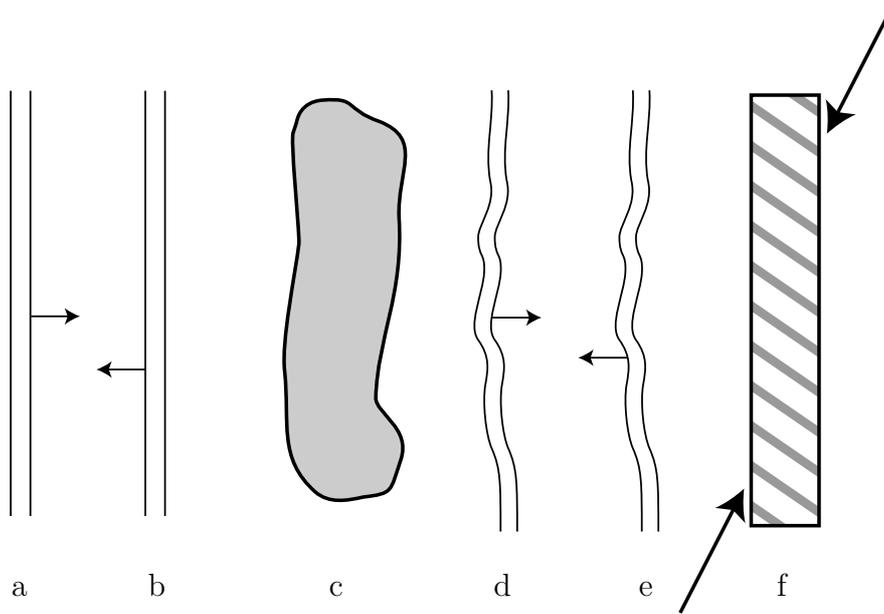
**Figure 9:** The phase conjugate mirror. An incident wave (a) encounters an obstacle (c), whereupon the wavefront is distorted (d). Two strong, counterpropagating beams, create a standing wave pattern in the nonlinear material (f), which is experienced as a grating by the incident weak beam. The resulting reflected wave (e) has exactly the same wave front as the incident wave, but is propagating in the opposite direction. After passing through the distorting medium, the wave front is restored.
