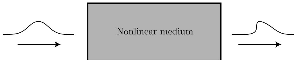
**Figure 10:** The profile of a pulse changes as it propagates through a nonlinear medium. This can be used to create strong pulses with short rise-time.
