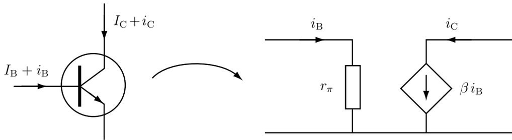
**Figure 4:** A small signal scheme modeling a transistor. The total base current is  $I_B + i_B$ , where the bias current  $I_B$  is much larger than the signal current  $i_B$ . The total collector current  $I_C + i_C$  is similarly decomposed. The amplification factor  $\beta$  and the resistance  $r_\pi$  in the scheme for the signal currents  $i_B$  and  $i_C$  depend on  $I_B$ .
