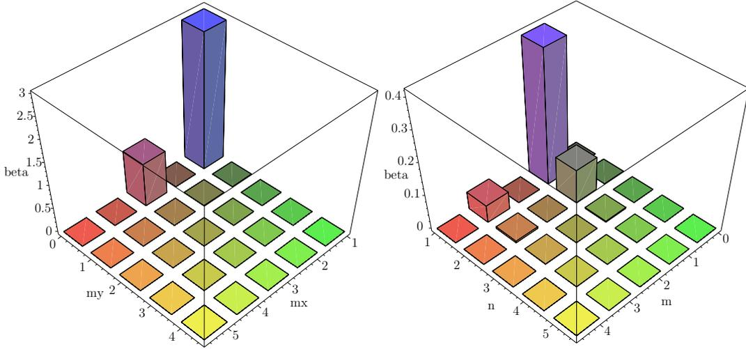
**Figure 3:** The distribution of the amplitude of the coupling factor  $|\beta_{um}|$  for a waveguide with rectangular (left) and circular (right) cross section. The index  $m$  is in both cases composed of two indices ( $m_x$  and  $m_y$  for the rectangular waveguide, and  $m$  and  $n$  for the circular). The tall bars correspond to  $\alpha_{u1}$ .
