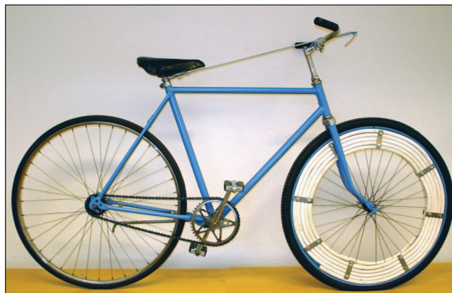
Figure 14. The Lund University bicycle. This bicycle has a weighted front wheel to exaggerate gyroscopic effects and an elastic cord attached to a neck on the front fork to enhance self-stabilization.
