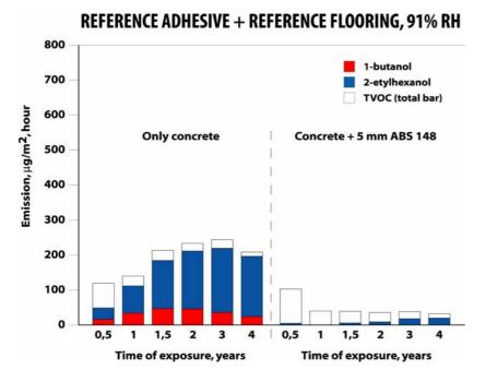
**Figure 5**. Emissions from composite structures on concrete with water/binder ratio = 0.7 and 91% RH (measured half a year after the application of the flooring)
