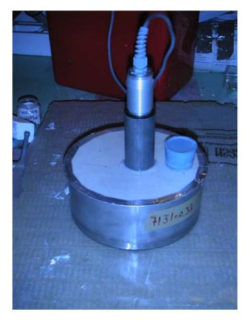
Figure 2. Set-up for measuring the relative humidity under the flooring.
