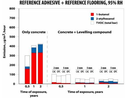
**Figure 7**. Emissions from composite structures on concrete with water/binder ratio = 0.62 and 95% RH (measured half a year after the application of the flooring). Reference flooring system. Levelling compound CAC has only calcium aluminate cement, while levelling compound OPC has a combination of ordinary Portland cement and calcium aluminate cement.
