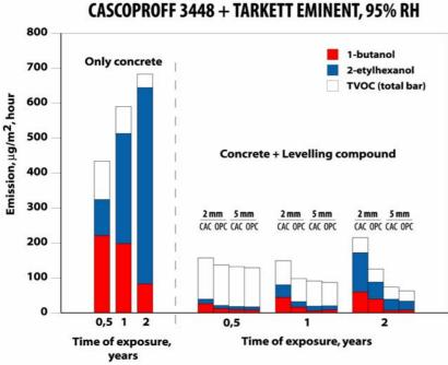
**Figure 8**. Emissions from composite structures on concrete with water/binder ratio = 0.62 and 95% RH (measured half a year after the application of the flooring). Commercial flooring system. Levelling compound CAC has only calcium aluminate cement, while levelling compound OPC has a combination of ordinary Portland cement and calcium aluminate cement.
