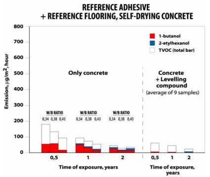
**Figure 9**. Emissions from composite constructions on self-desiccating concrete with different water/binder ratios. The results with levelling compound are the average of 9 samples.
