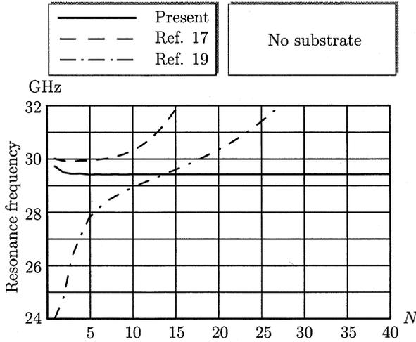
Fig. 9. Resonance frequency versus the number of Floquet modes included for the tripole array of Fig. 6 but without the dielectric substrate. The angles of incidence are  $\theta = 45^\circ$  and  $\phi = 90^\circ$ .
