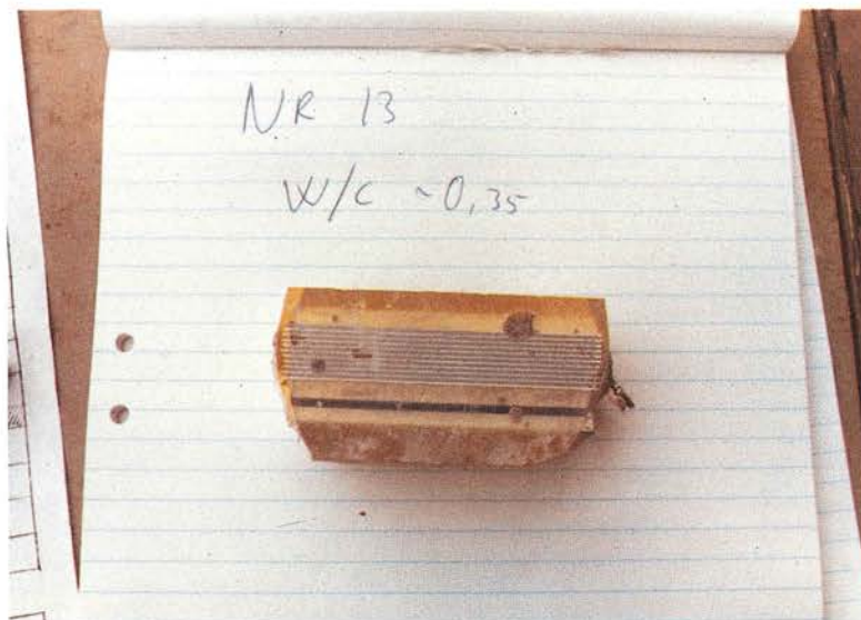
Photo 29. Corrosion cell where about 20% of the anodic area has begun to corrode. Note that the three steel plates show no more than local corrosion. Cell No. 13, in Series 2.
