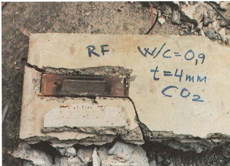
Photo 32. Corrosion cell in Series 3, KC6-78 which had been in carbonated concrete and then been subjected to wetting to study the cell current as a function of the relative humidity and temperature.
