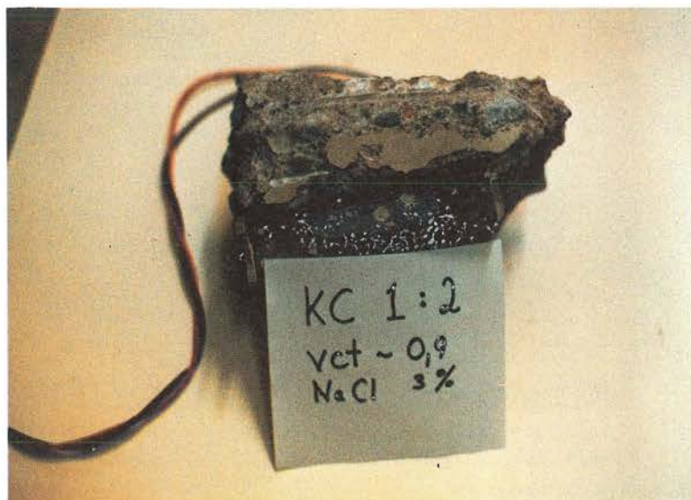
Photo 10. Corrosion cell after exposure to a 3% NaCl solution for about 60 days. A large quantity of corrosion products can be seen with the naked eye on the entire cell, particularly on the anodic areas. Concrete quality KC1-76, W/C approx. 0.8, concrete cover 7 mm.
