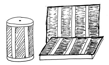
Inside the cups and bags are placed portions of silicagel to accumulate the moiture and keep the air dry. A measuring of the relative humidity inside shows RH=7-13%. The following results of the vapour resistance are based on calculations with 10% RH.
