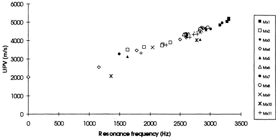
Figure 7: Resonance frequency vs. pulse velocity in ASTM C666 procedure A. 11 concretes up to maximum 300 cycles, max 10 measurements per series, mean of three beams pr serie, 62 sets of data.  $UPV = 1.10 \cdot frequ + 1418$ ,  $r = 0.96$
