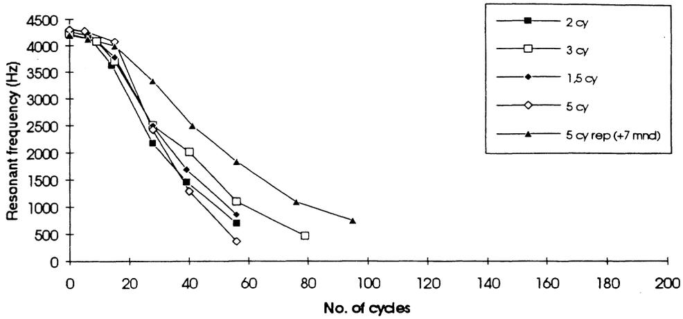
Fig. 7: Resonance frequency vs. number of cycles, 040-05
