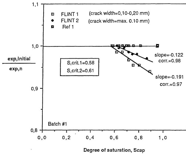
Fig. 3. Diagram showing the critical degree of saturation ( $S_{crit.}$ ) from freeze-thaw testing of samples in batch 1. The amount of expansion and the expansion rate (steepness of curves) is increasing with increasing crack width.
