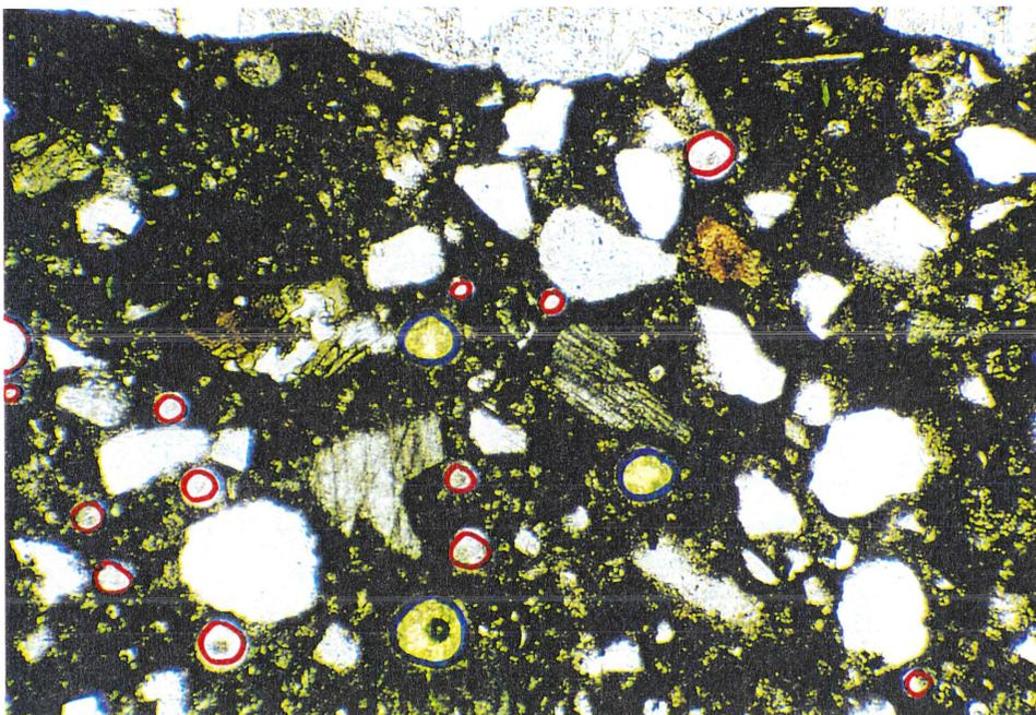
*Fig. 5. Site 55. An air-entrained concrete where the original air content has been high but where most of the air pores in the field of micrograph are filled with ettringite. There has been 16 air pores in the area of the micrograph, of which only 3 are still open (marked with a blue circle). 13 pores have been filled with ettringite (marked with red circle). The height of the micrograph is about 1 mm.*
