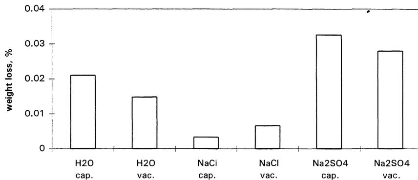
Fig. 3. Weight loss, expressed in percent of original weight, of granite after 35 cycles of freeze-thaw in pure water and 2% salt solutions of NaCl and  $\text{Na}_2\text{SO}_4 \cdot 10 \text{H}_2\text{O}$ . The specimen were either capillary (cap.) or vacuum (vac.) saturated.
