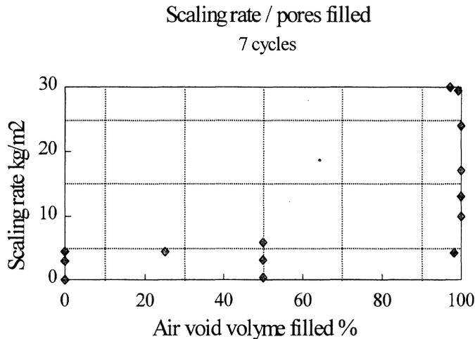
Figure 2. *Pore void filling and the freeze/thaw durability of the same type of concrete. The scaling rate is high if the pores are filled with secondary reaction products. The freeze/thaw scaling rate is rather independent of the original air content.*
