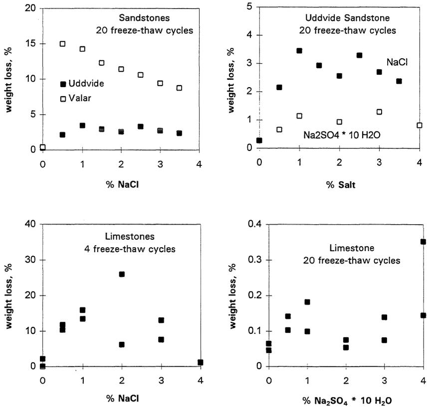
Fig. 2. Weight loss, expressed in percent of original weight, after freezing and thawing of sandstones and limestone in NaCl- and  $\text{Na}_2\text{SO}_4$ -solutions of different concentrations. Note the different scales on the y-axes.
