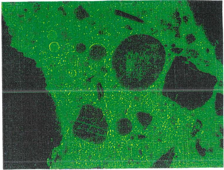
*Picture 3. The same specimen in fluorescent light. The fluorescent epoxy does not penetrate the "round aggregates" or the natural aggregates because both these do have a very dense structure. The size of the photographed area is about 0.8 mm x 1.3 mm.*
