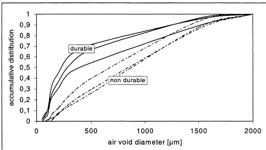
Figure 5. Accumulative distribution versus air void diameter.
