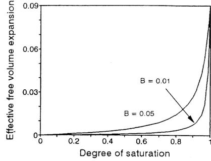
Fig. 3. Effective free volume expansion as function of degree of saturation<sup>1</sup>.  $B$  expresses the deviation from pure cylindrical pores (Figure 1).
