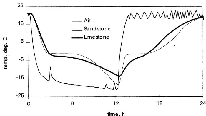
Fig. 1. Freeze-thaw cycle used in the scaling test.
