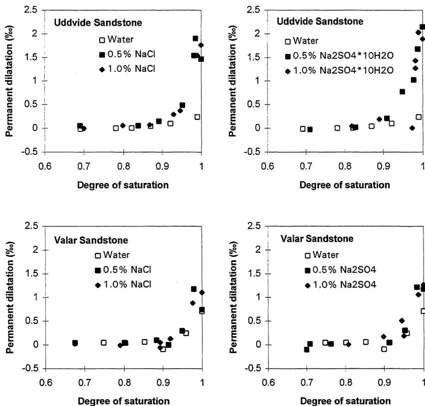
Fig. 5. Permanent dilatation after one freeze-thaw-cycle of sandstones as function of the degree of saturation of NaCl- and Na<sub>2</sub>SO<sub>4</sub>-solutions of different concentrations.
