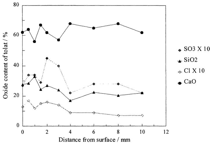
Figure 1. *The changes in the chemical composition of the paste during the freeze/thaw cycles at the laboratory test. Chlorides are penetrating in to the concrete and the close to the surface calcium is leached out.*
