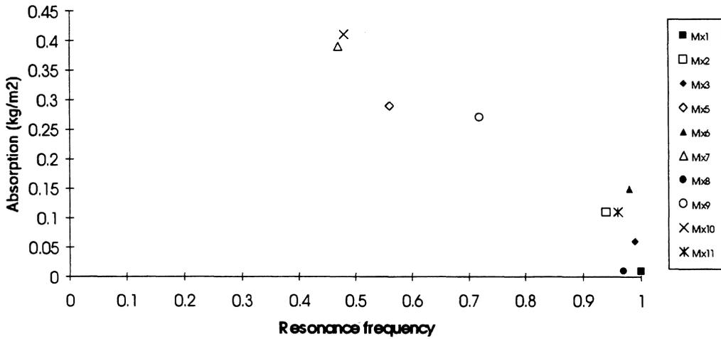
Figure 6: Resonance frequency (normalized to initial value) vs. absorption 70 cycles
