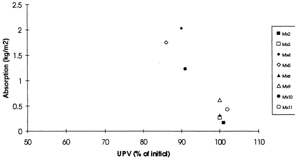
Figure 5: Pulse velocity vs. absorption after 56 cycles in SS 13 72 44.
