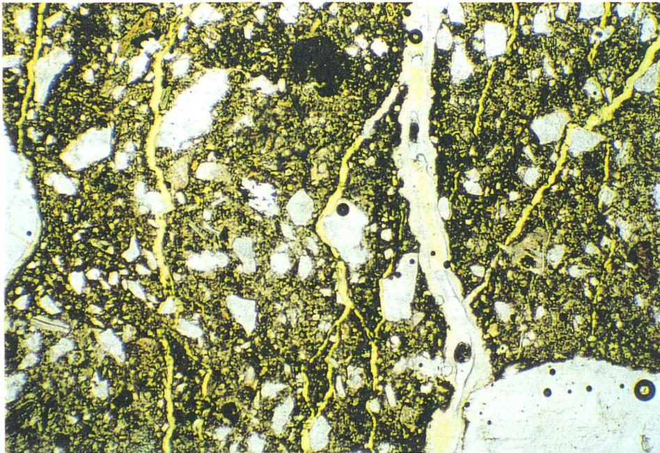
*Fig. 7. Site 6. Frost damages in the concrete. The facade has been impregnated. The resin has filled the broadest crack and partly some minor cracks branch out of it. The height of the micrograph is 2,8 mm.*
