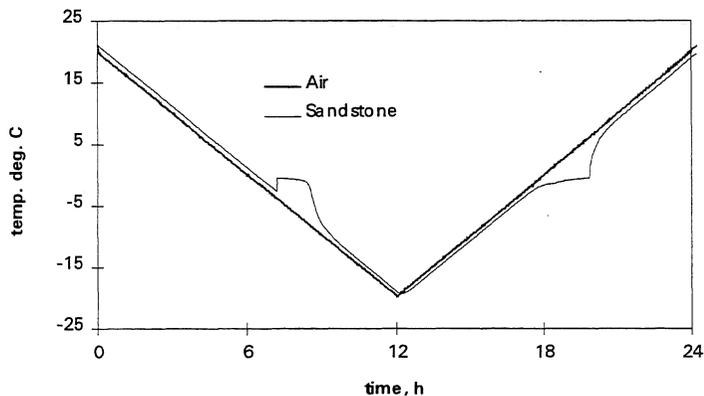
Fig. 4. Freeze-thaw -cycle used in the dilatation test.
