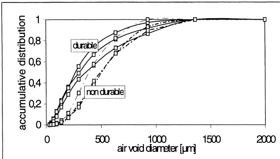
Figure 2. Accumulative distribution versus air void diameter.
