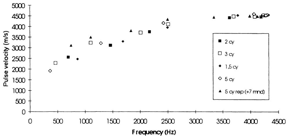
Fig. 9: Resonance frequency vs. pulse velocity for 040-05
