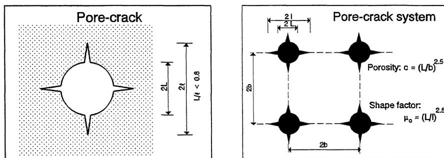
Fig. 1. System of pore-cracks (spherical or cylindrical voids) used in the model. Fracture mechanics can be used when  $L/l < 0,8$ .
