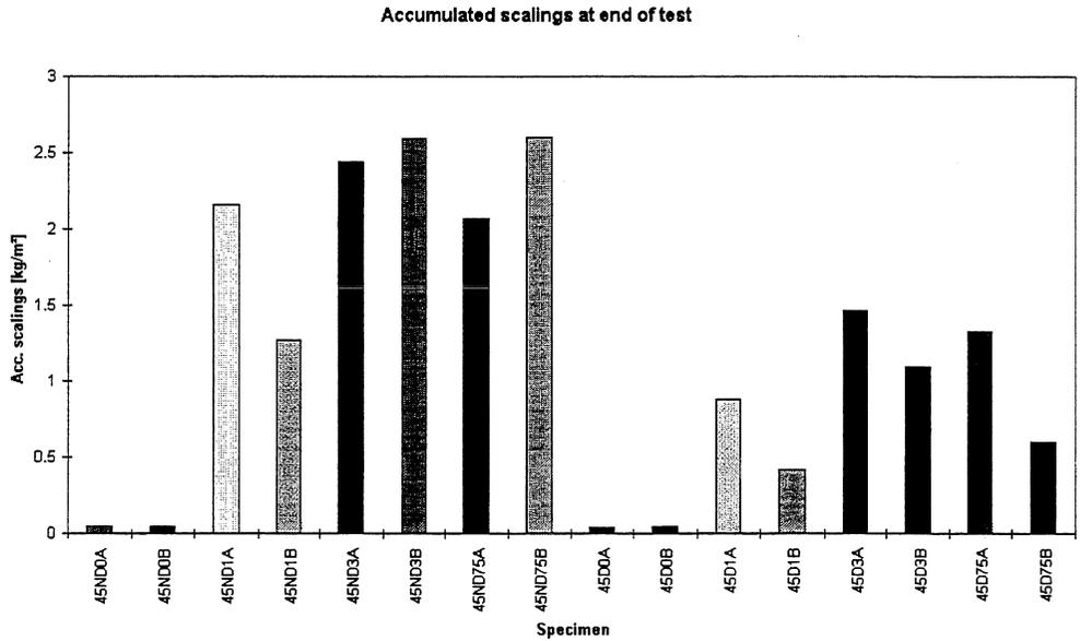
*Fig 7: Final accumulated scalings (W/C 0.45, 10 cycles)*
