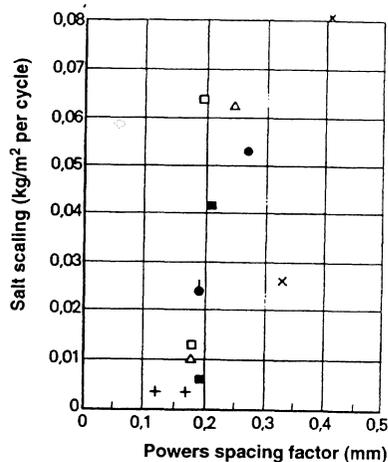
Figure 5: Experimental determination of the salt scaling resistance versus the Powers spacing factor; /13/.
