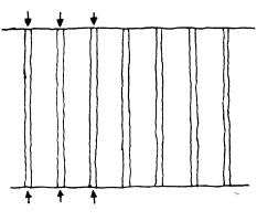
As we in the right case above have lines of symmetry (small arrows) we can simplify the problem even further, by looking only at that part of a flow path that is between two margo strands (including half a strand at each side). We then get a 2-dimensional diffusion problem in a plane perpendicular to the strands. Below are two drawings of this:
