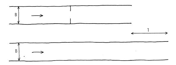
Both these structures give the same resistance to flow (i.e. give the same flow with the same gradient). In the top case the obstruction gives an extra resistance. In the bottom case the lengtening gives the same extra resistance.
