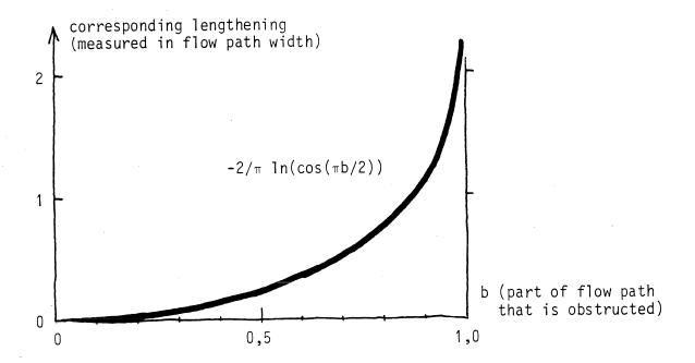
The distance between the margo strands is (calculated from Bolton and Petty 1978) 0,25  $\mu m$  for earlywood and 0,4  $\mu m$  for latewood. The strand thicknesses are 0,03  $\mu m$  amd 0,1  $\mu m$ . This means that 12% and 25% respectively are blocked (b=0,12 and 0,25). As we can see in the diagram the extension of the flow path corresponding to this is negligeble.
