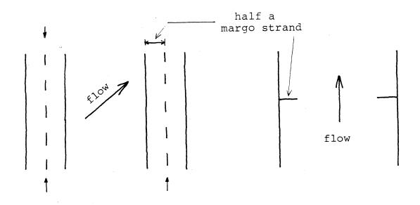
We need only consider half the structure, as the flow after the margo obstruction is a mirror image of the flow before the obstruction (B is the width of the flow path and b is the part of it that is blocked).
