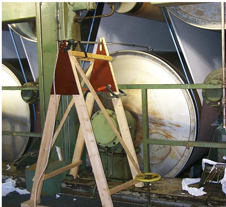
Figure 5.1 The temperature measuring equipment mounted at cylinder 33.
