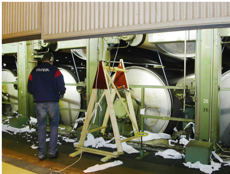
Figure 3.1 The dryer section just after a web break. The paper is on the floor instead of on the cylinders.
