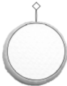
Figure 9 A plasterboard sample with wax sealing and a circle describing the estimated area. (Paper III)
