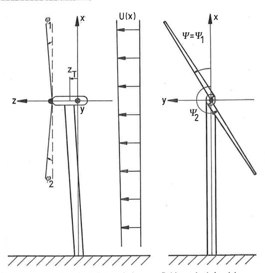
Figure 3.1: A schematic picture of the wind turbine.
