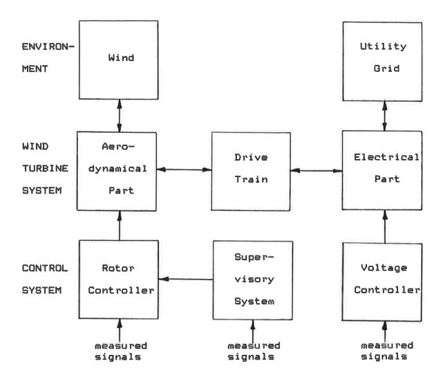
Figure 2.1: The structure of the wind turbine system.
