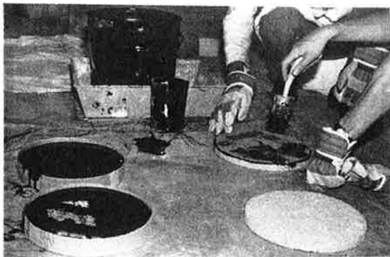
Fig. 4. Left: Oxidized bitumen (proposal 2). Right: Brushing out the membrane of proposal 1.
