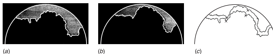
Figure 7. Formaldehyde LIF signal images detected at (a) -2 CAD and (b) -0.5 CAD. The identified contours have been superimposed on both images. (c) The two contours illustrated together. The corresponding points given as input for velocity calculation are indicated with \times -marks.
