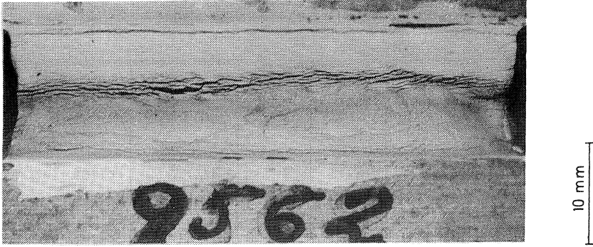
FIG. 5.9 Photo of specimen No. 9562 after 39 months of outdoor exposure. The specimen has been elongated 10.1% and compressed 22.4% (cf. Table 5.8).
