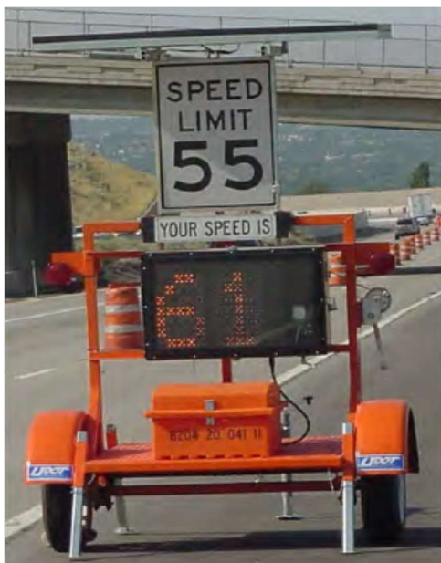
Figure 13. Speed Monitoring Display (Bowie, 2003).
