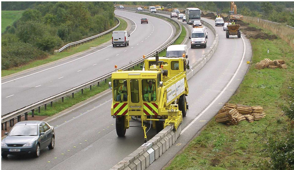
Figure 23. A “Quick moveable barrier” ( http://www.barriersystemsinc.com/stuff/contentmgr/files/0/06bcc8d5b07bf7de9c026797c585635/files/qmb_const_pi_sheet_international_04_18_13.pdf )
