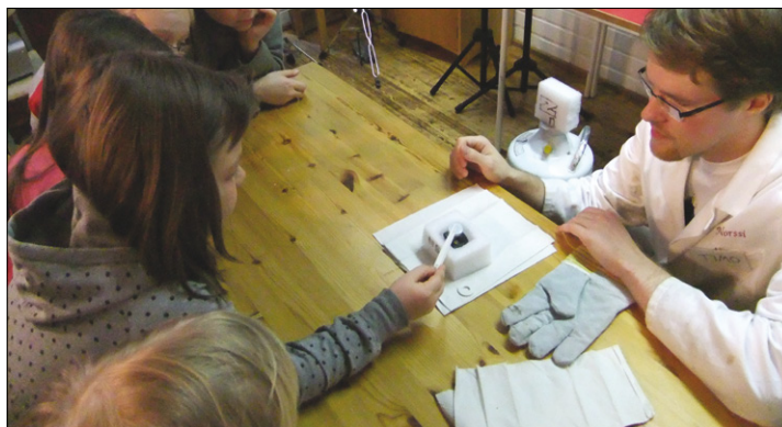
The magnet hovers over a cooled superconductor and won't budge.
