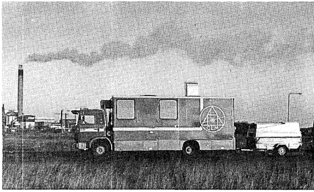
Fig. 1. Mobile remote sensing laboratory with its motor generator trailer.
