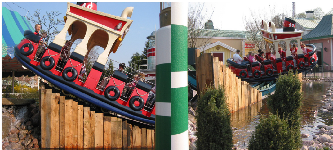
Figure 1. The Rockin' Tug family ride combines a pendulum and circular motion. The little tug moves back and forth along a circular rail and at the same time rotates along its own axis orthogonal to the rail.
