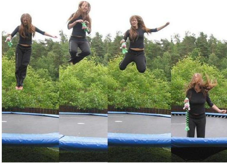
Figure 1. A spiral toy used as accelerometer during a trampoline jump. Note how the spiral in the toy is contracted while the jumper is in the air, and expanded at the bottom of the jump. Also note how far down the trampoline is displaced in the last photo.
